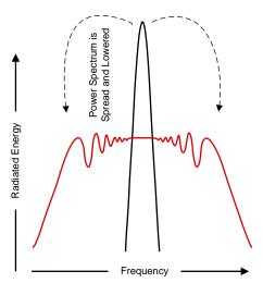
Where a fixed frequency converter exhibits large amounts of spectral energy at the switching frequency, the spread spectrum architecture of the LP8732xx-Q1 spreads that energy over a large bandwidth.
