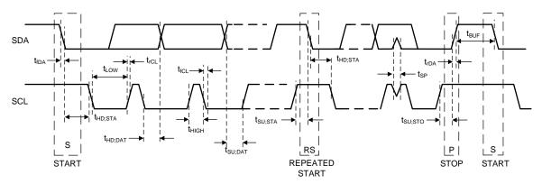
Figure 25. I<sup>2</sup>C-Compatible Timing
