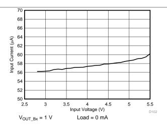
Figure 3. Active State Current Consumption vs Input Voltage, One Buck Regulator Enabled in PFM Mode (singlephase)
