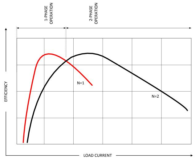
Figure 9. Multiphase Buck Converter Efficiency vs Number of Phases. All Converters in PWM mode. (UPDATE) (1)
