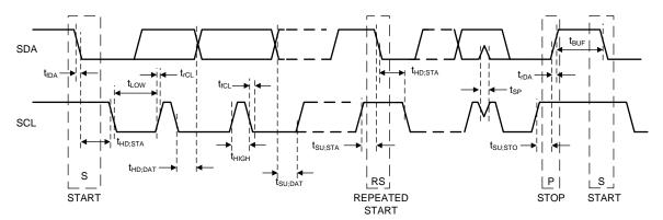
Figure 1. I<sup>2</sup>C Timing
