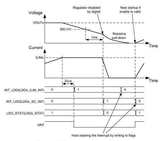
Figure 21. LDO Regulator Overload Situation
