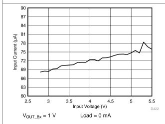
Figure 4. Active State Current Consumption vs Input Voltage, Regulator Enabled in PFM Mode (dual-phase)
