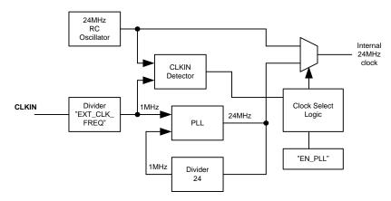
Figure 12. Clock and PLL Module
