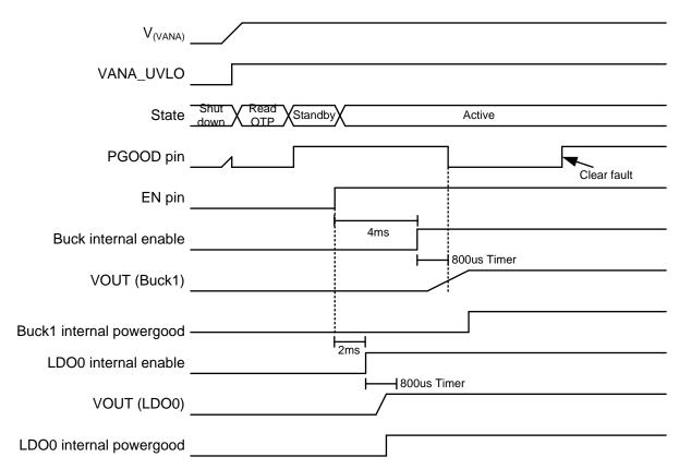
Figure 17. PGOOD Pin Operation in Gated Mode
