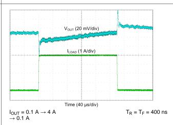
Figure 65. Buck Transient Load Step Response, Forced PWM Mode (Dual-Phase Output)
