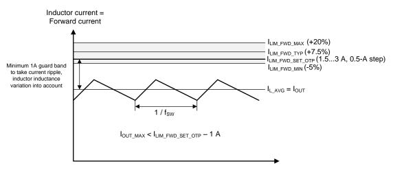
Figure 31. Current Limit vs Maximum Output Current
