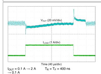
Figure 62. Buck Transient Load Step Response, AUTO Mode (Single-Phase Output)
