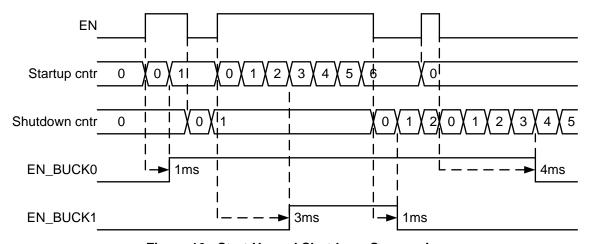
Figure 16. Start-Up and Shutdown Sequencing
