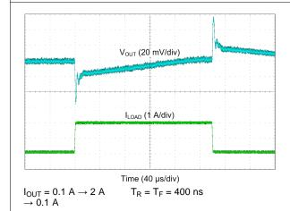
Figure 64. Buck Transient Load Step Response, Forced PWM Mode (Single-Phase Output)
