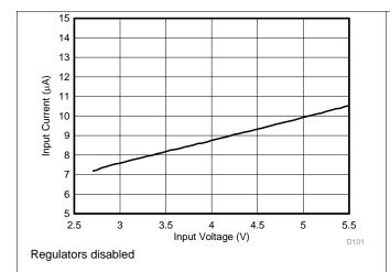
Figure 2. Standby Current Consumption vs Input Voltage
