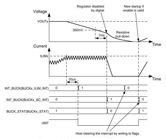
Figure 20. Buck Regulator Overload Situation
