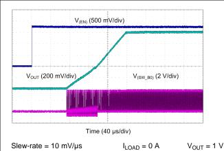
Figure 46. Buck Start-Up With EN1, Forced PWM Mode (Single-Phase Output)
