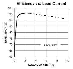
Figure 1. Efficiency Curve
