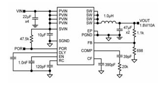
MIC22950 10A Synchronous DC-DC Converter
