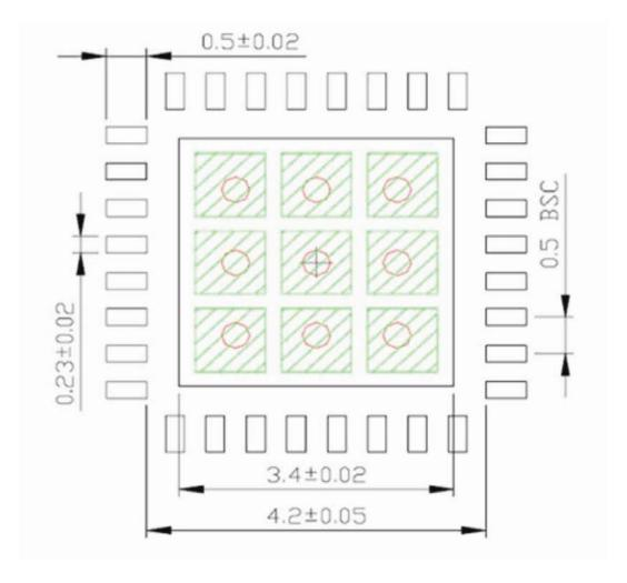
Red circle indicates Thermal Via. Size should be 300 – 350mm in diameter, 1.00mm pitch, and it should be connected to GND plane for maximum thermal performance.
