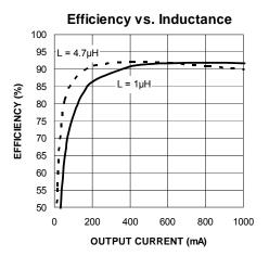
Figure 2. Efficiency vs. Inductance
