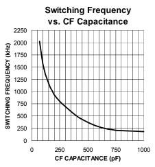
Figure 3. Switching Frequency vs. CF Capacitance
