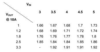
Table 1. Power Dissipation (W) for 10A Output
