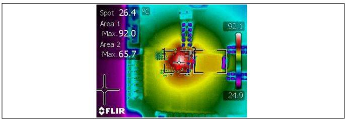
Figure 22 Thermal image of the board at 25 A load TDA38827 = 92°C, L = 65.7°C, fsw = 800 kHz, room temperature, natural convection
