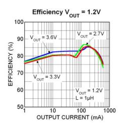
Figure 1. MIC23050 Efficiency Curve
