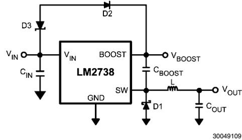
FIGURE 4. Zener Reduces Boost Voltage from  $V_{IN}$
