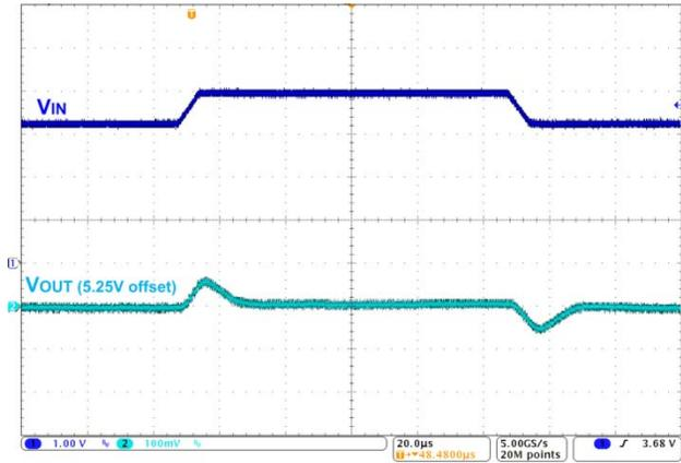
Figure 17. Line Transient, 3.2 <--> 3.9  $V_{IN}$ , 7  $\mu\text{s}$  Edge, 120 mA Load
