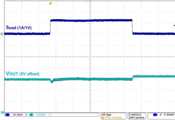
Figure 15. Load Transient, 0 <--> 120 mA, 1  $\mu\text{s}$  Edge
