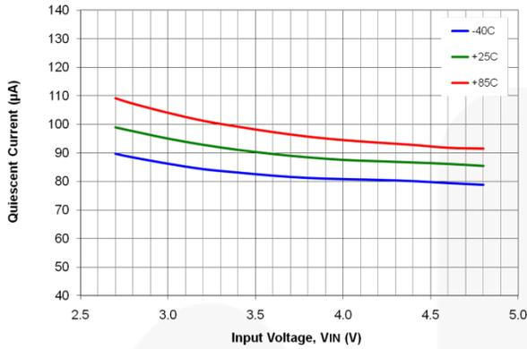
Figure 5. Quiescent Current vs. Input Voltage and Temperature
