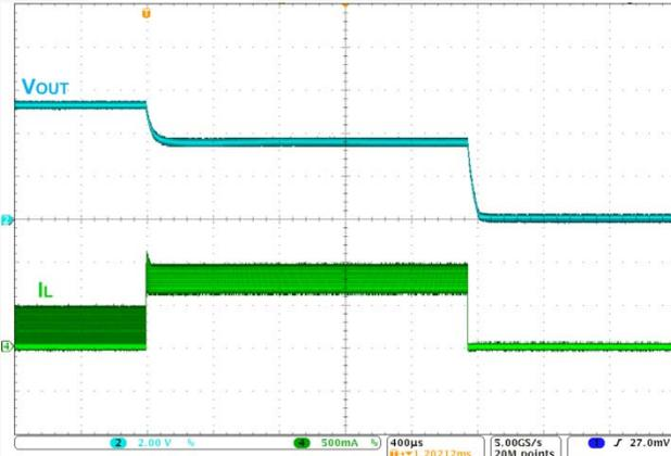
Figure 14. Overload Protection
