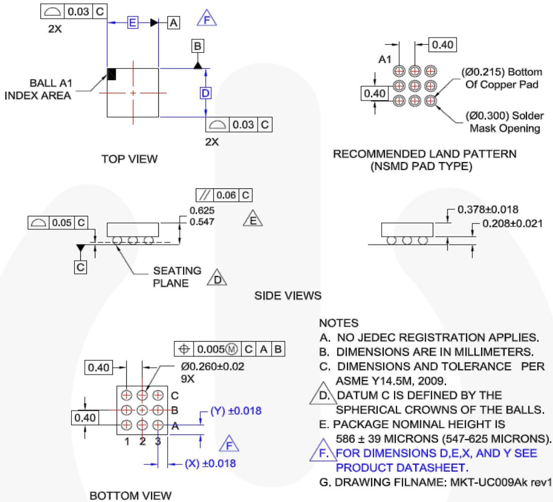
Figure 20. 9-Bump, 0.4 mm Pitch, Wafer-Level Chip-Scale Package (WLCSP)
