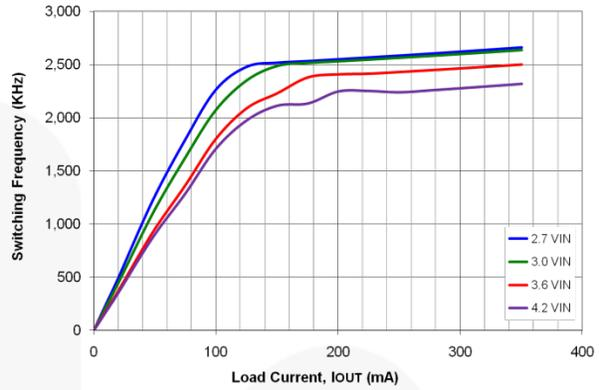
Figure 12. Switching Frequency vs. Load Current and Temperature
