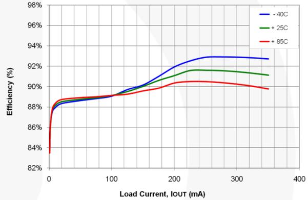
Figure 8. Efficiency vs. Load Current and Temperature
