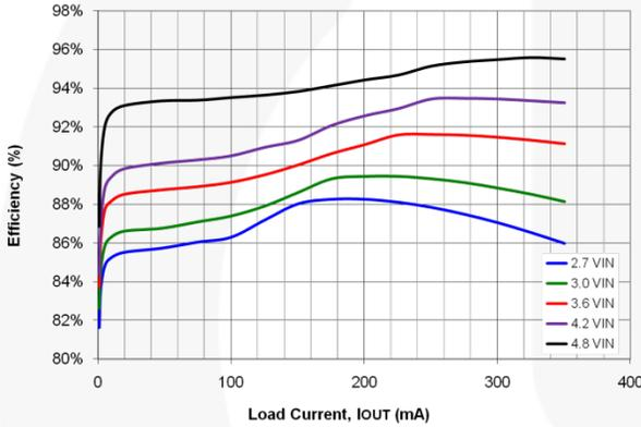
Figure 7. Efficiency vs. Load Current and Input Voltage
