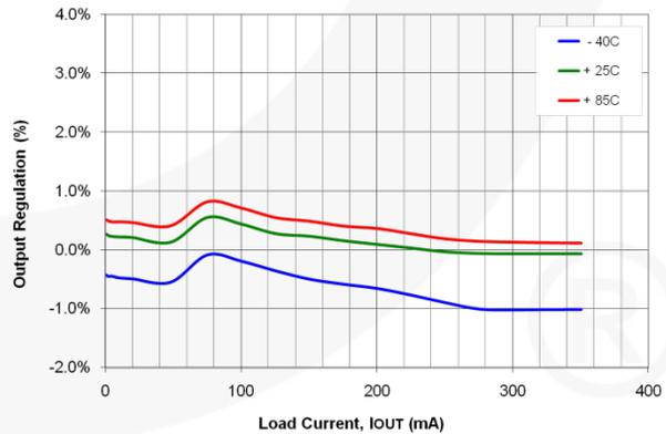
Figure 10. Output Regulation vs. Load Current and Temperature
