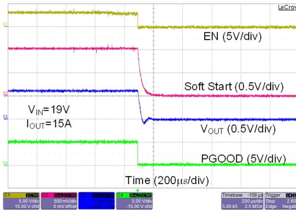
**Figure 18. Shutdown Waveforms with 15 A Load Current**
