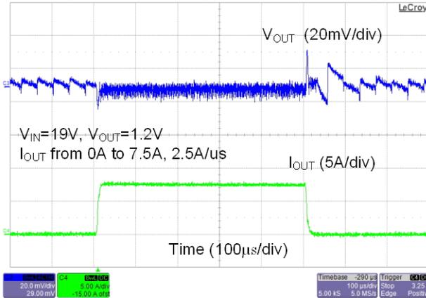
**Figure 24. Load Transient from 0% to 50% Load Current**
