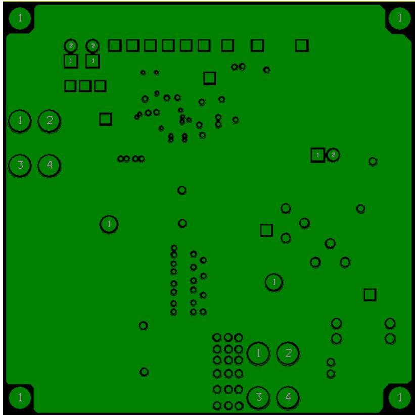
Figure 30. Evaluation Board Inner Layer 2 Copper
