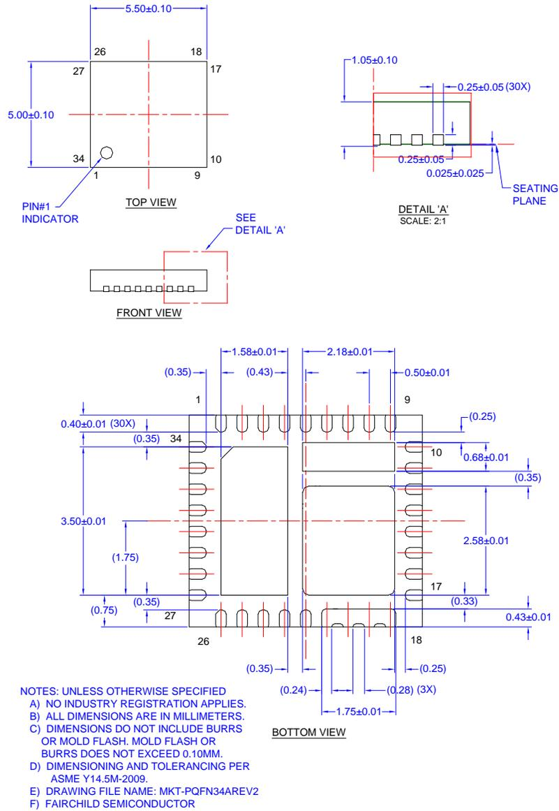
**Figure 32.34-Lead, PQFN, 5.5 mm x 5.0 mm Package**
