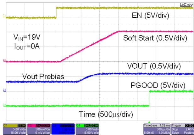
**Figure 19. Startup Waveforms with Pre-Bias Voltage on Output**
