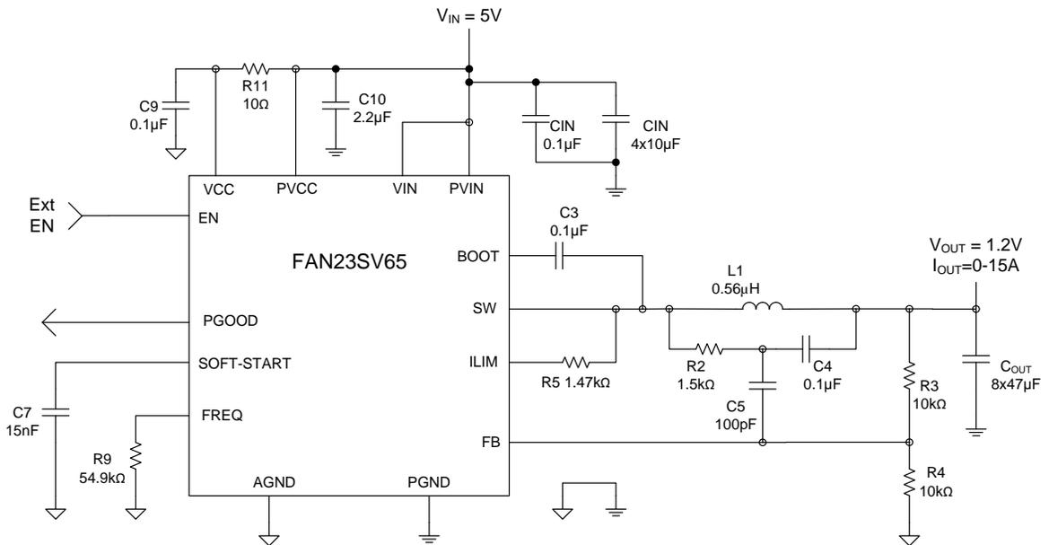
Figure 2. Typical Application with  $V_{IN} = 5V$
