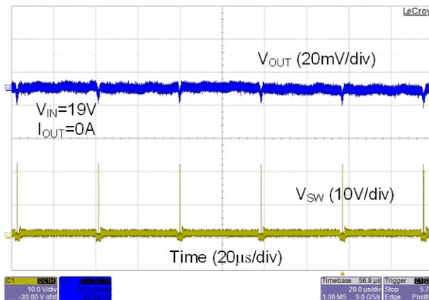
**Figure 20. Static Load Ripple at No Load**
