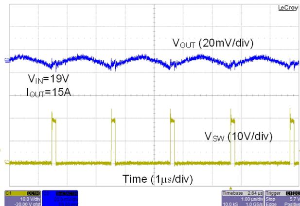
**Figure 21. Static Load Ripple at Full Load**
