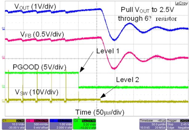
**Figure 27. Over-Voltage Protection Level 1 and Level 2**
