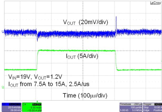
**Figure 25. Load Transient from 50% to 100% Load Current**
