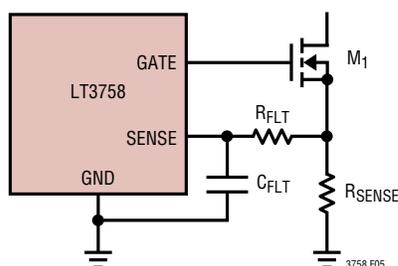
Figure 5. The RC Filter on the SENSE Pin
