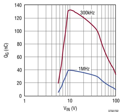
Figure 2. Recommended Maximum Q<sub>G</sub> vs V<sub>IN</sub> at Different Frequencies to Ensure INTV<sub>CC</sub> Higher Than 4.7V
