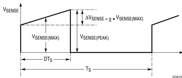
Figure 4. The Sense Voltage During a Switching Cycle
