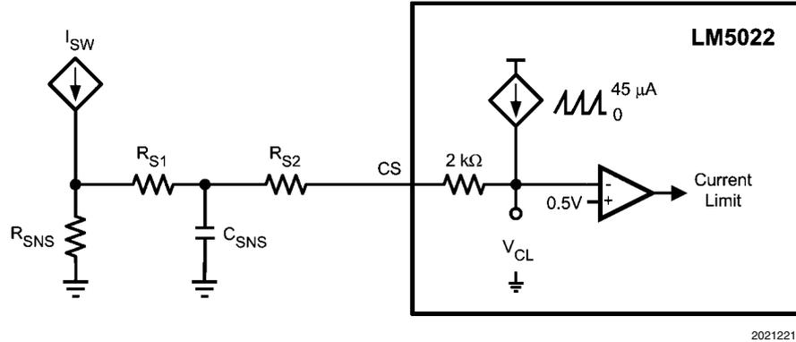
FIGURE 4. Slope Compensation
