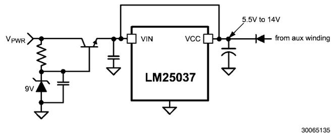
FIGURE 11. Start-up Regulator for  $V_{PWR} > 75V$
