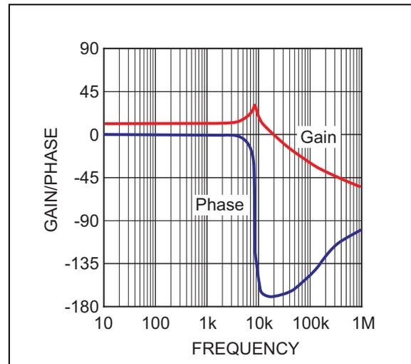
**FIGURE 4-25:**  $G_{VD}$  Transfer Function.
