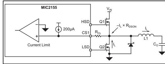
FIGURE 4-13: Overcurrent Detection Circuit.
