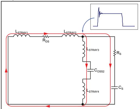
**FIGURE 4-23:** Snubber Circuit.
