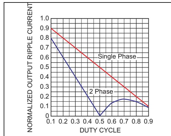
**FIGURE 4-19:** Phase Output Ripple Current vs. Duty Cycle.
