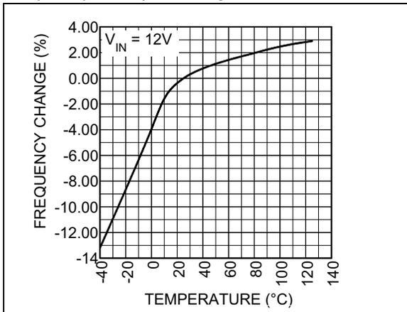
**FIGURE 2-8:** Change in Switching Frequency vs. Temperature.
