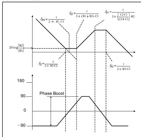
**FIGURE 4-26:** Type III Compensated Error Amplifier Gain/Phase.
