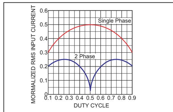
**FIGURE 4-21:** RMS Input Current vs. Duty Cycle.
