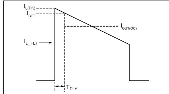
**FIGURE 4-15:** Overcurrent Waveform.
