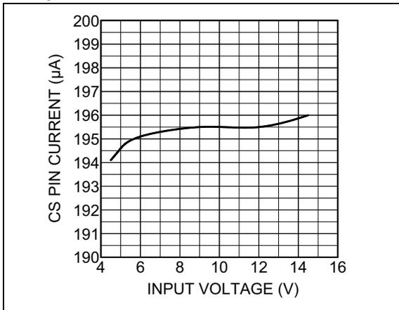
**FIGURE 2-14:** CS Pin Current vs. Input Voltage.
