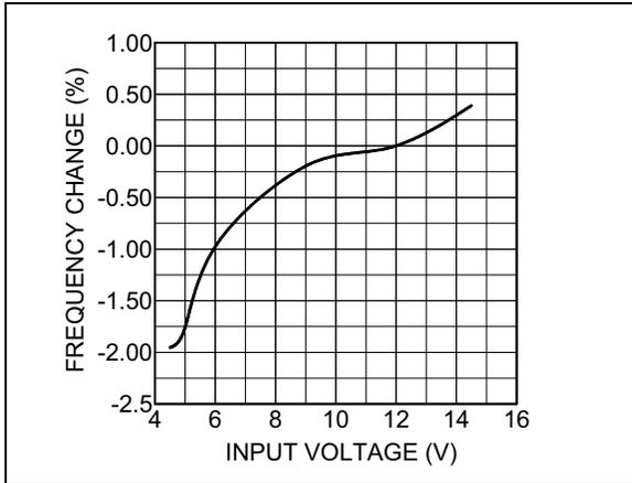
**FIGURE 2-7:** Change in Switching Frequency vs. Input Voltage.
