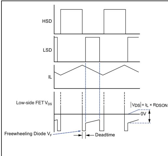
**FIGURE 4-14:** Inductor Current and Low-Side FET  $V_{DS}$  Waveforms.
