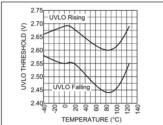
**FIGURE 2-2:** VIN2 UVLO Threshold.
