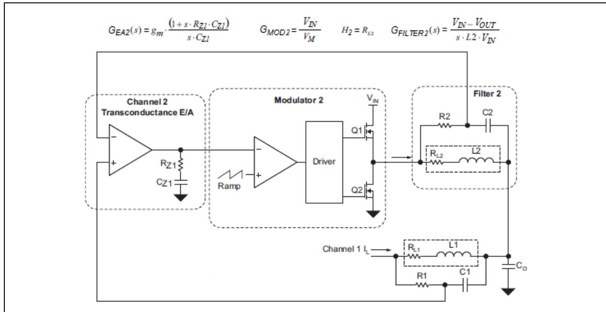
**FIGURE 4-27:** Current Sharing Loop and Transfer Functions.
