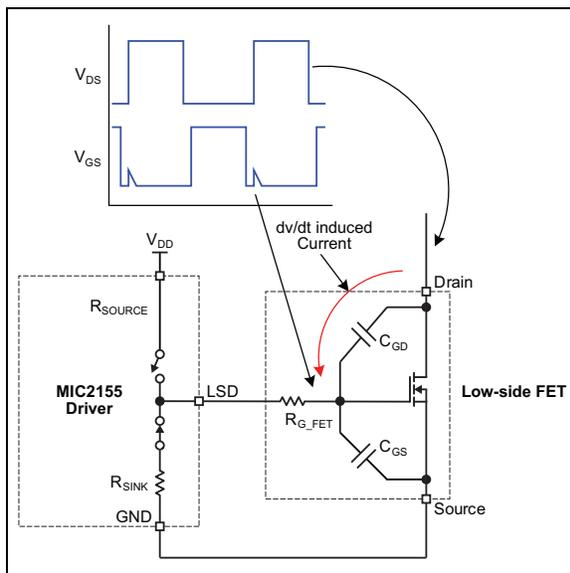
**FIGURE 4-10:** *dv/dt-Induced Turn-on.*
