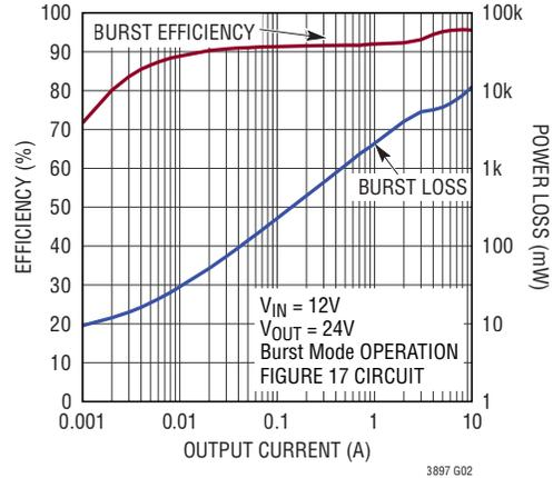
**Efficiency vs Input Current**
