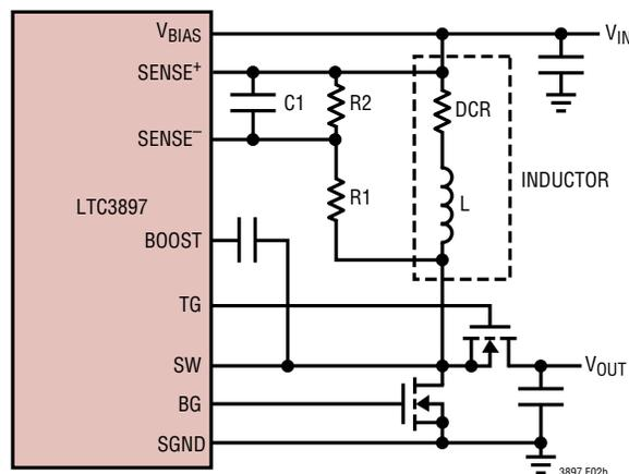
PLACE C1 NEAR SENSE PINS  $(R1 || R2) \cdot C1 = \frac{L}{DCR}$   $R_{SENSE(EQ)} = DCR \cdot \frac{R2}{R1 + R2}$
