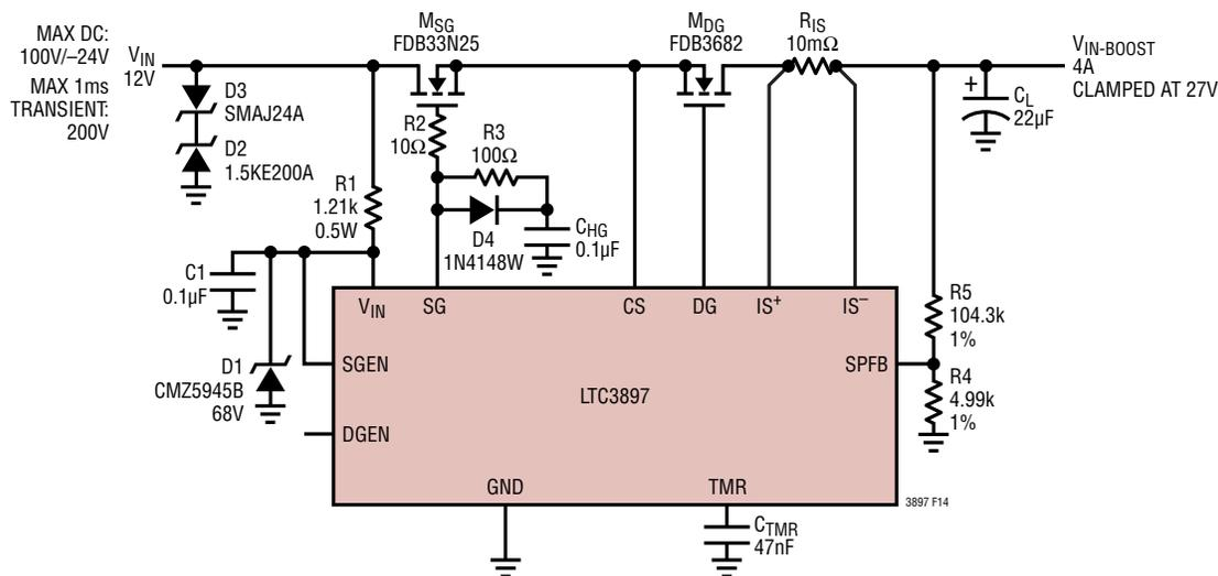
Figure 14. 4A, 12V Overvoltage and Reverse Current Protection
