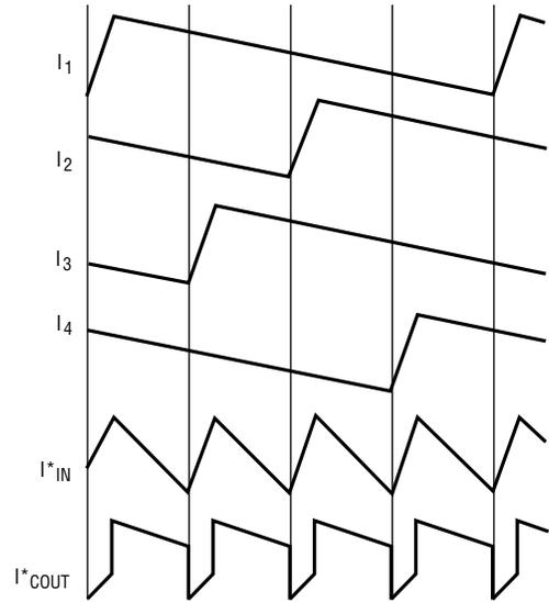
\* RIPPLE CURRENT CANCELLATION INCREASES THE RIPPLE FREQUENCY AND REDUCES THE RMS INPUT/OUTPUT RIPPLE CURRENT, THUS SAVING INPUT/OUTPUT CAPACITORS
