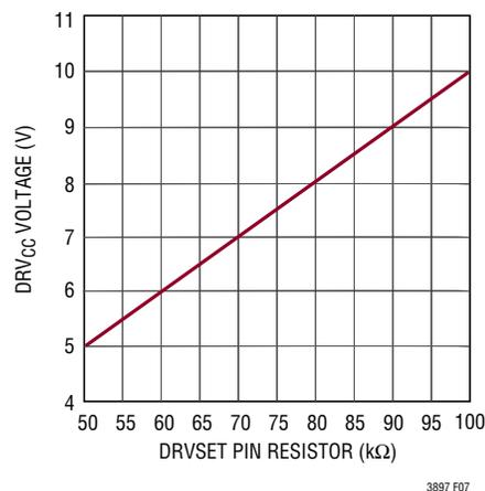
Figure 7. Relationship Between DRV<sub>CC</sub> Voltage and Resistor Value at DRVSET Pin
