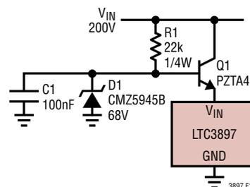
Figure 11. Buffering  $V_{IN}$  to Extend Input Supply Range
