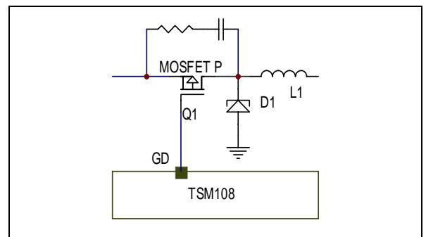
The RC components should realise a time constant corresponding to one tenth of the switching time constant of the TSM108 (i.e. in our example, the oscillator frequency is set to 10µs corresponding to 100kHz, therefore, the RC couple should realise a time constant close to 1µs).
