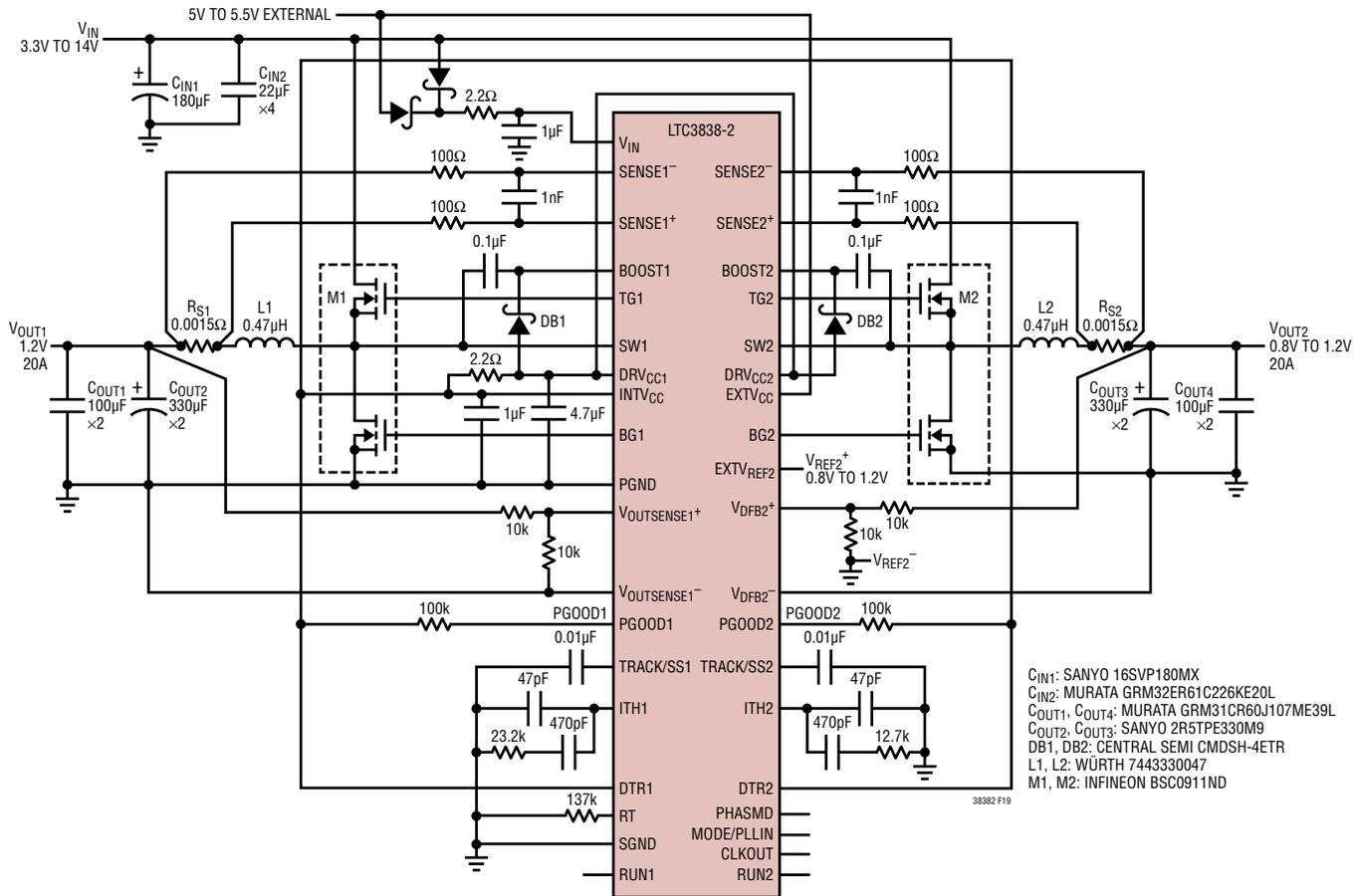
**Note:** When operating with the power  $V_{IN}$  supply below 5.5V, this application requires the 5V to 5.5V external supply to be present at  $EXTV_{CC}$  in order to maintain  $DRV_{CC}$ ,  $INTV_{CC}$  and  $V_{IN}$  pin voltages needed for the IC to function properly. The  $EXTV_{CC}$  supply is optional when the power  $V_{IN}$  supply is at or above 5.5V.
