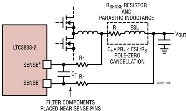
Figure 3a. R<sub>SENSE</sub> Current Sensing
