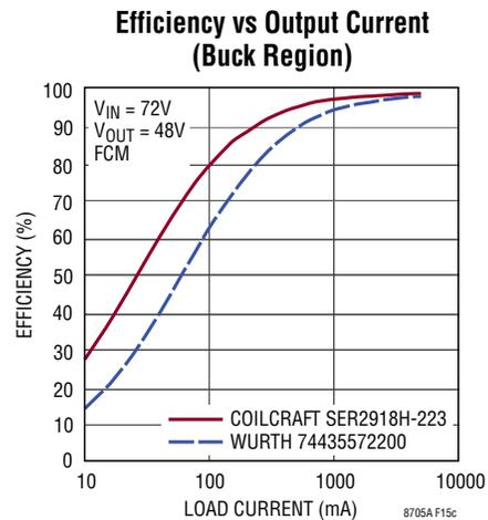
Note: See the front page and the Typical Performance Characteristics section for more curves from this application circuit using the Coilcraft inductor. The smaller Würth inductor is also suitable in place of the Coilcraft inductor with some loss in efficiency.
