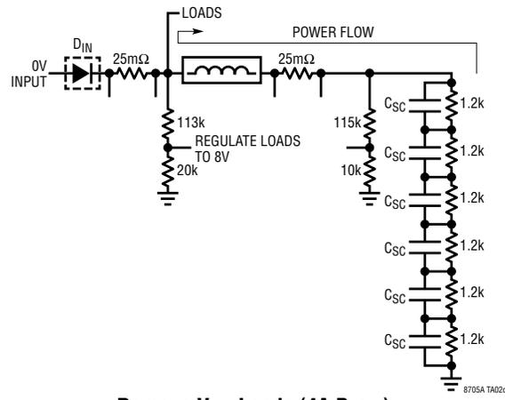
**Charging V<sub>OUT</sub> to 15V with 1A Current**
