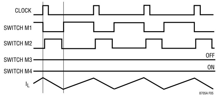
Figure 5. Buck Region ( $V_{IN} \gg V_{OUT}$ )
