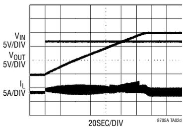
**Remove V<sub>IN</sub>. Loads (4A Draw) Regulated to 8V from Supercaps**
