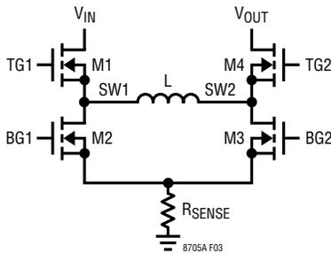
Figure 3. Simplified Diagram of the Output Switches
