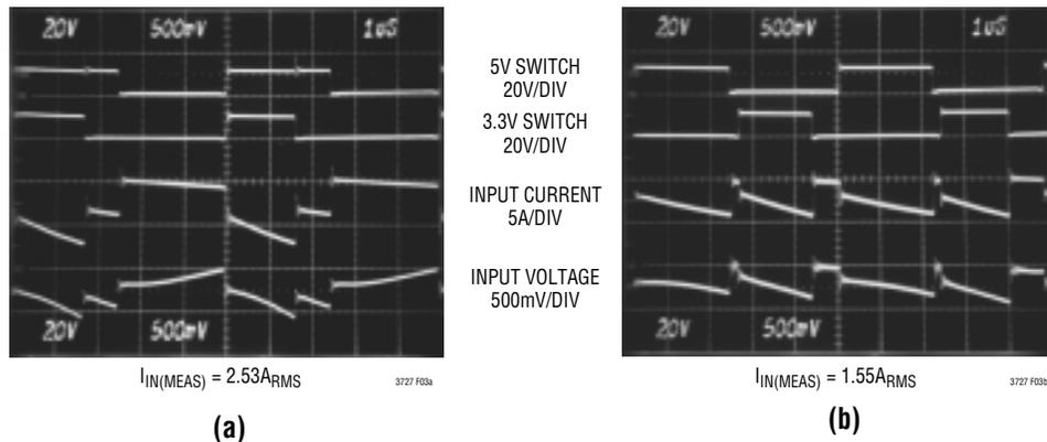
**Figure 3. Input Waveforms Comparing Single-Phase (a) and 2-Phase (b) Operation for Dual Switching Regulators Converting 12V to 5V and 3.3V at 3A Each. The Reduced Input Ripple with the LTC3727 2-Phase Regulator Allows Less Expensive Input Capacitors, Reduces Shielding Requirements for EMI and Improves Efficiency**
