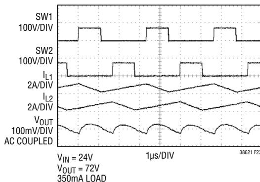
Figure 23. Switching Waveforms for a Boost Converter
