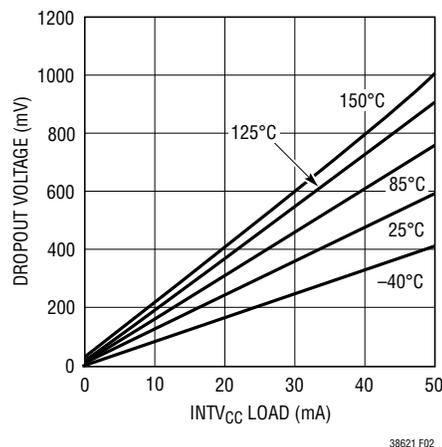
Figure 2.  $INTV_{CC}$  LDO Dropout Voltage vs Current
