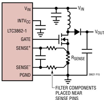
Figure 15. Proper Current Sense Filter Component Placement
