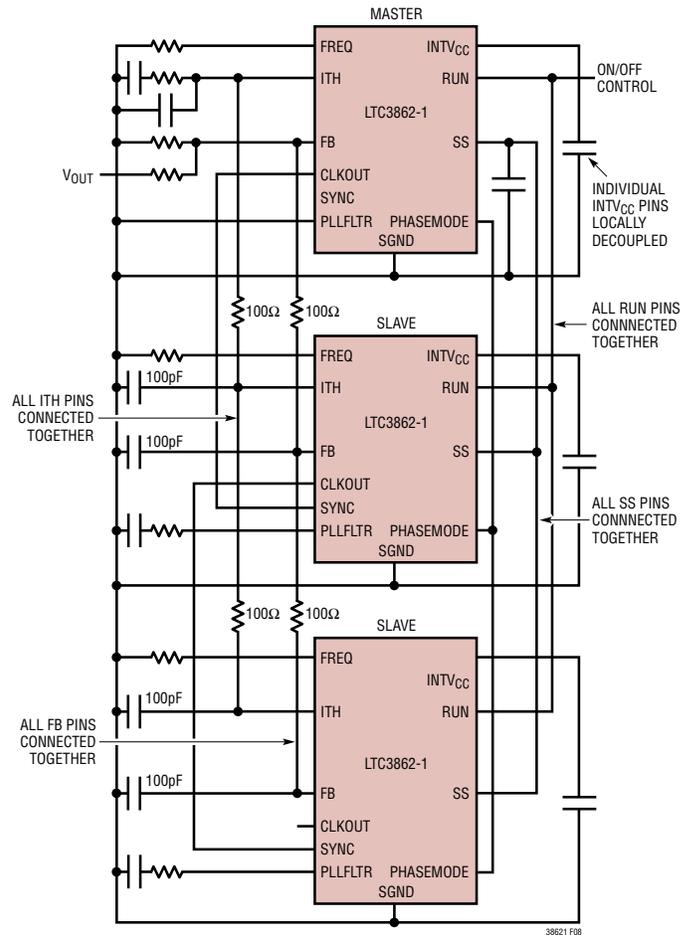
Figure 8. LTC3862-1 Error Amplifier Configuration for Multi-Phase Operation
