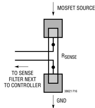
Figure 16. Connecting the SENSE<sup>+</sup> and SENSE<sup>-</sup> Traces to the Sense Resistor Using a Kelvin Connection
