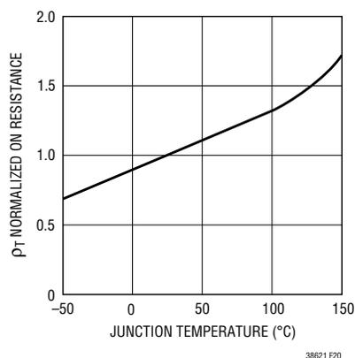
Figure 20. Normalized Power MOSFET  $R_{DS(ON)}$  vs Temperature
