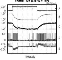
A: GATE, 5V/div D: LX1, 10V/div B: REFIN1, 0.5V/div E: INDUCTOR CURRENT, 5A/div C: OUT1 (1.0V TO 1.5V), 0.5V/div 200mA LOAD, SKIP = GND
