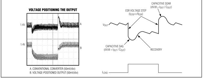
Figure 11. Voltage-Positioning Transient Response
