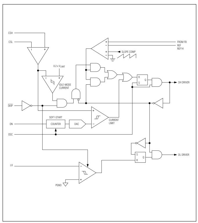
Figure 3. PWM-Comparator Functional Diagram
