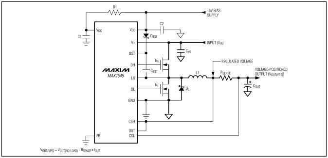
Figure 10. Voltage-Positioned Applications Circuit
