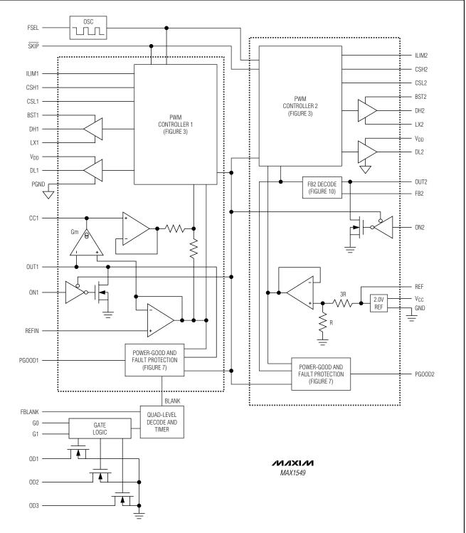
Figure 2. PWM-Controller Detailed Functional Diagram
