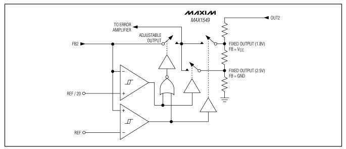
Figure 5. Second Controller's Dual-Mode Feedback
