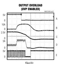
A: I<sub>OUT2</sub> = 0 TO 4A, 5A/div C: INDUCTOR CURRENT, 5A/div  $\frac{\text{B: V}_{0UT2} = 2.5\text{V}, 100\text{mV/div} \quad \text{D: LX2, 10V/div}}{\text{SKIP} = \text{V}_{CC}}$
