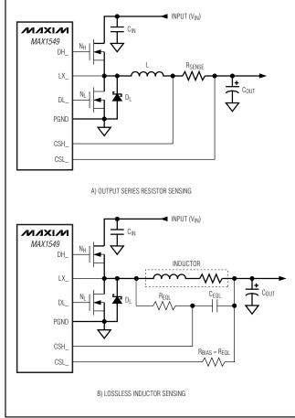
Figure 8. Current-Sense Configurations
