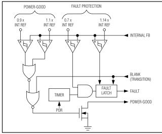
Figure 7. Power-Good and Fault Protection
