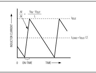
Figure 4. Pulse-Skipping/Discontinuous Crossover Point
