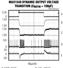
A: GATE, 5V/div D: LX1, 10V/div B: REFIN1, 0.5V/div E: INDUCTOR CURRENT, 10A/div C: OUT1 (1.0V TO 1.5V), 0.5V/div 200mA LOAD, SKIP = GND
