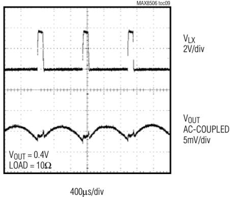
**LIGHT-LOAD SWITCHING WAVEFORM IN NORMAL MODE**
