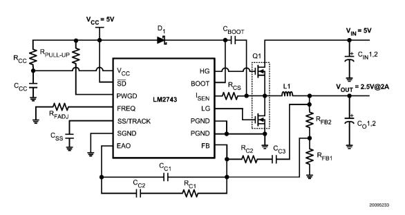
FIGURE 18. 5V to 2.5V @ 2A,  $f_{SW} = 300 kHz$
