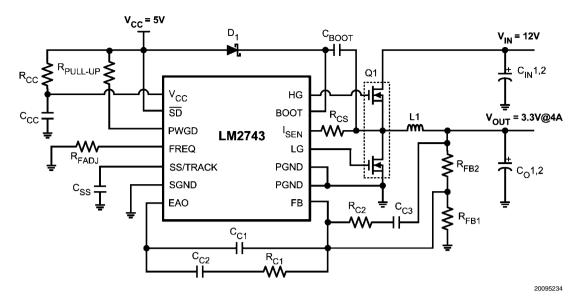
FIGURE 19. 12V to 3.3V @ 4A, f<sub>SW</sub> = 300kHz
