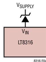
Figure 4. Increased Supply Voltage with a Zener Diode
