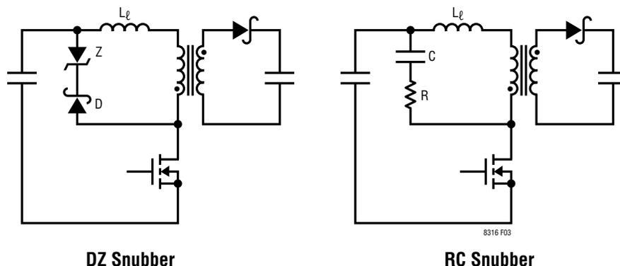
Figure 3. Snubber Circuits
