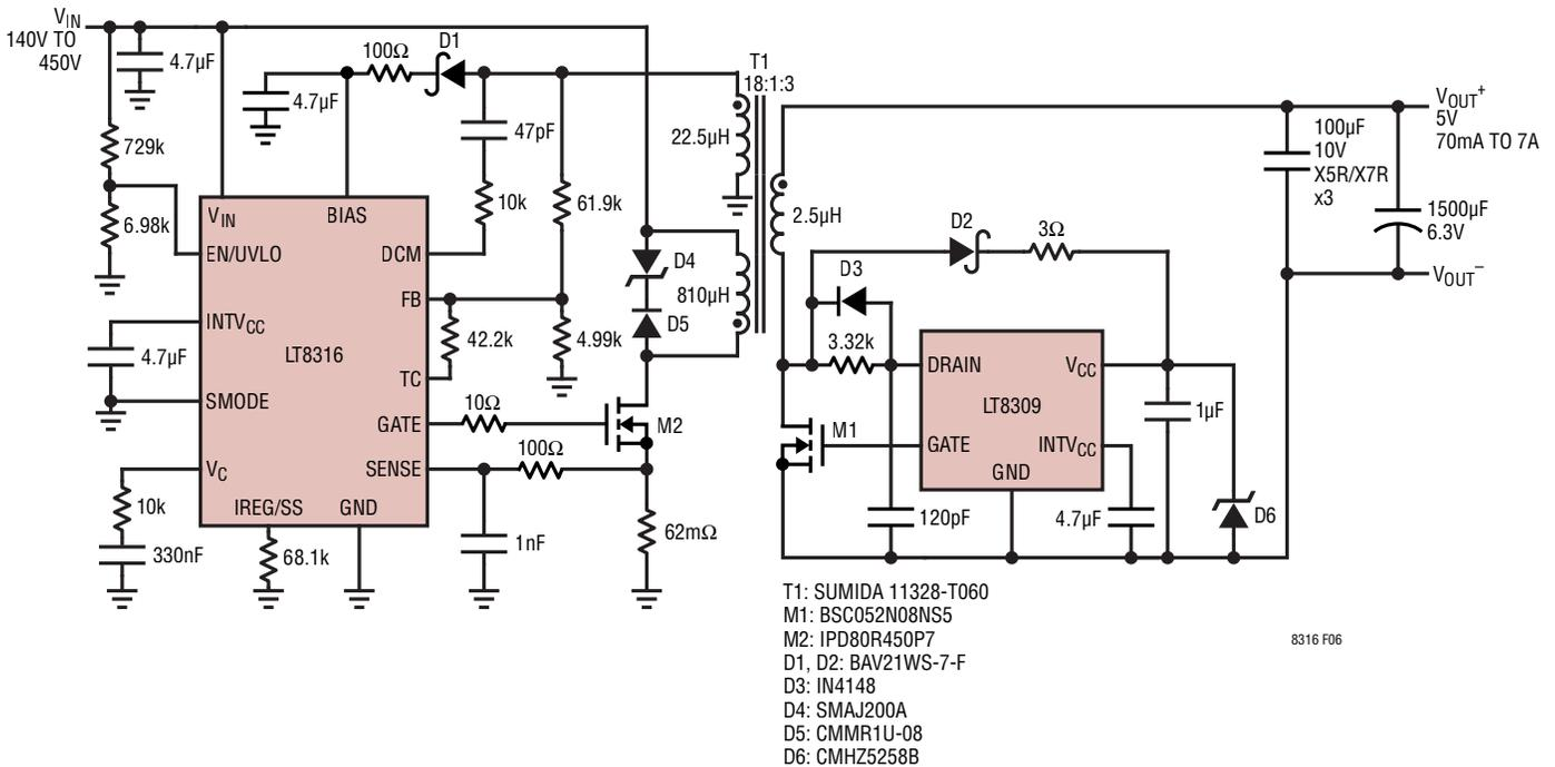
Figure 6. 91% Efficient Isolated 5V/7A Synchronous Flyback Converter
