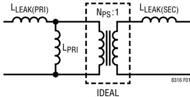
Figure 1. Transformer Model
