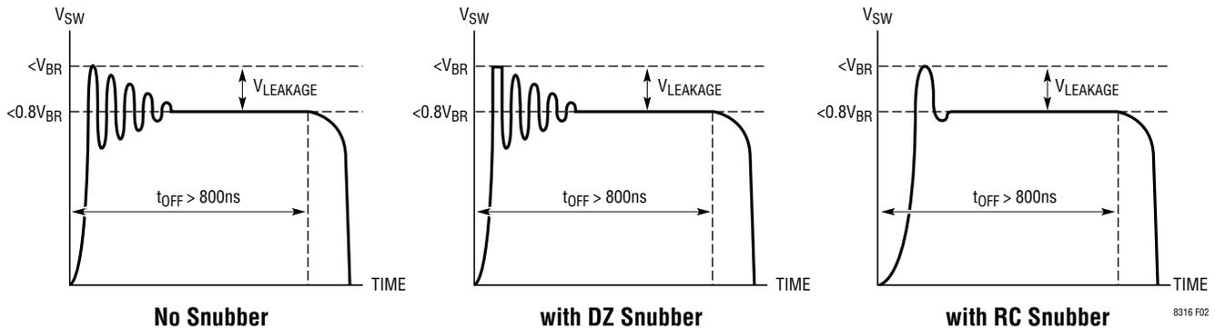
Figure 2. Maximum Voltages for SW Pin Flyback Waveform
