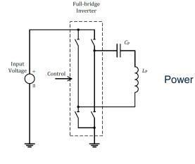
$Lp = 10 \pm 10\% \mu H$   $Cp = 247 \pm 5\% nF$  fop = 110 kHz to 145 kHzduty cycle of ton/tperiod = 5% to 50%.
