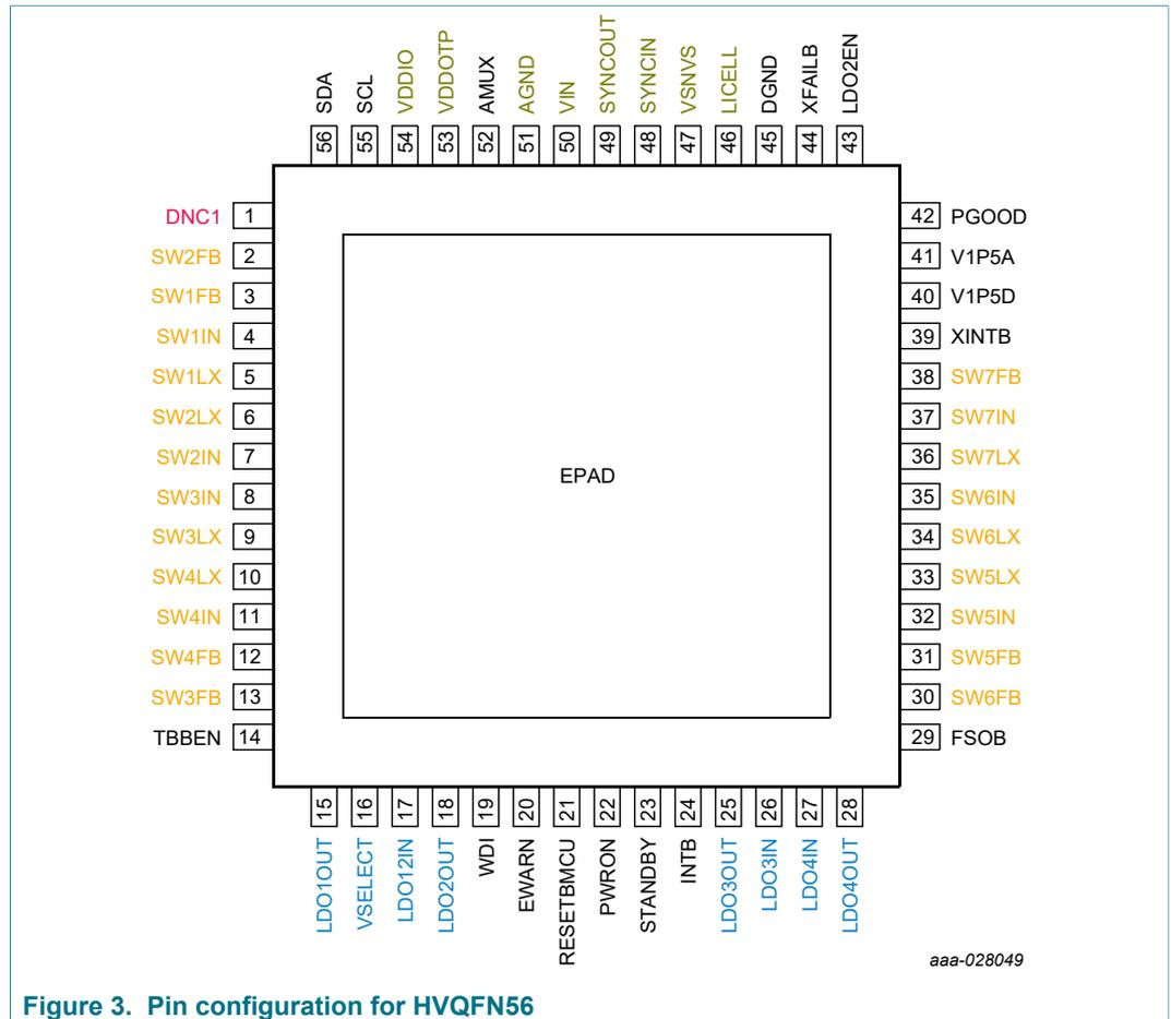
Figure 3. Pin configuration for HVQFN56
