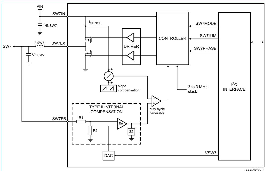
Figure 28. Type 2 buck regulator block diagram
