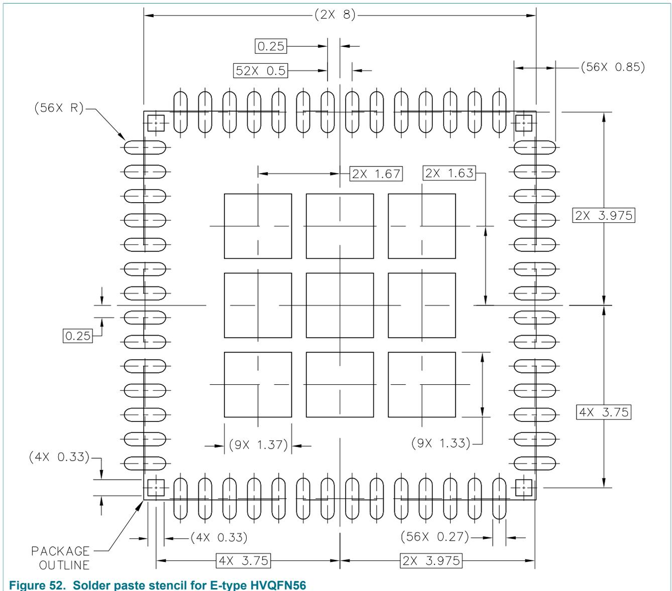
Figure 52. Solder paste stencil for E-type HVQFN56
