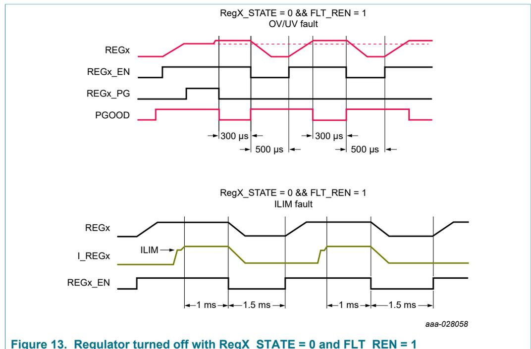
Figure 13. Regulator turned off with RegX\_STATE = 0 and FLT\_REN = 1
