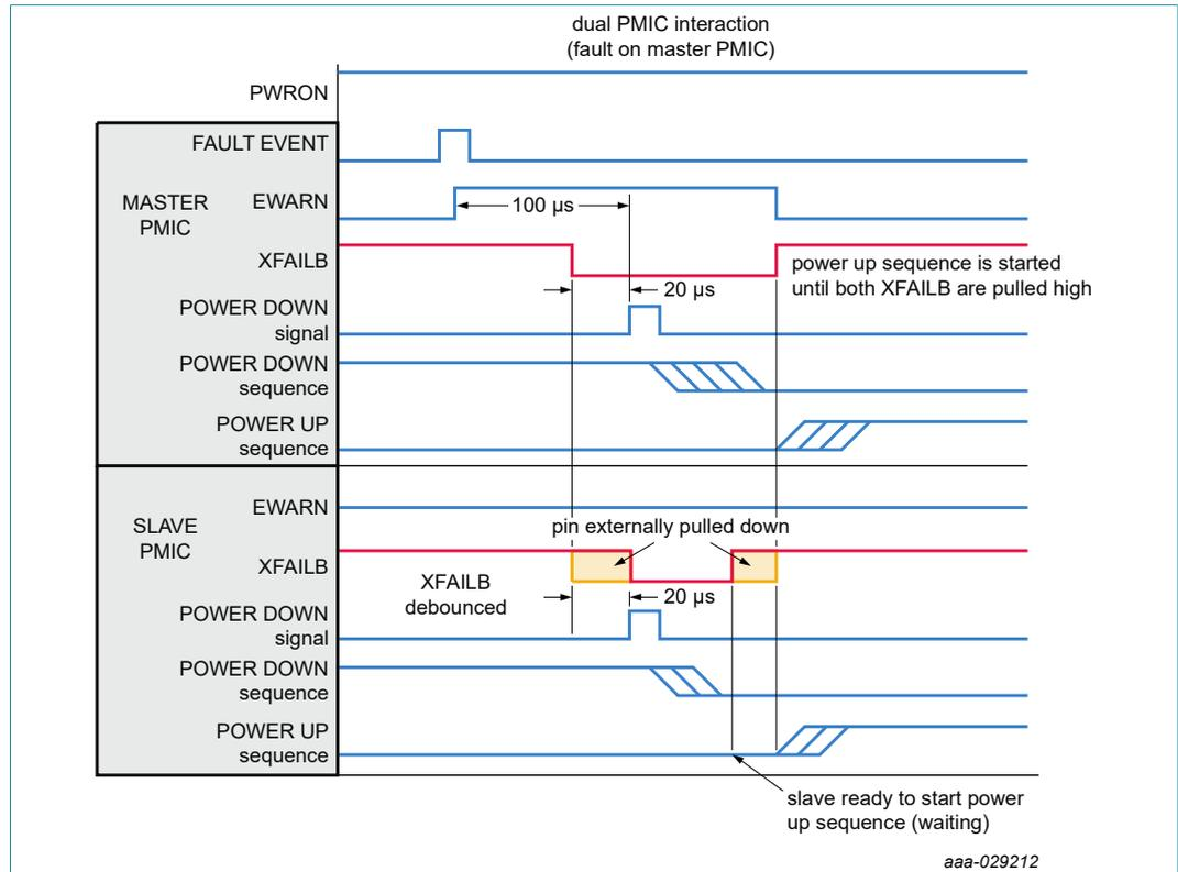
Figure 20. Behavior during an external XFAILB event
