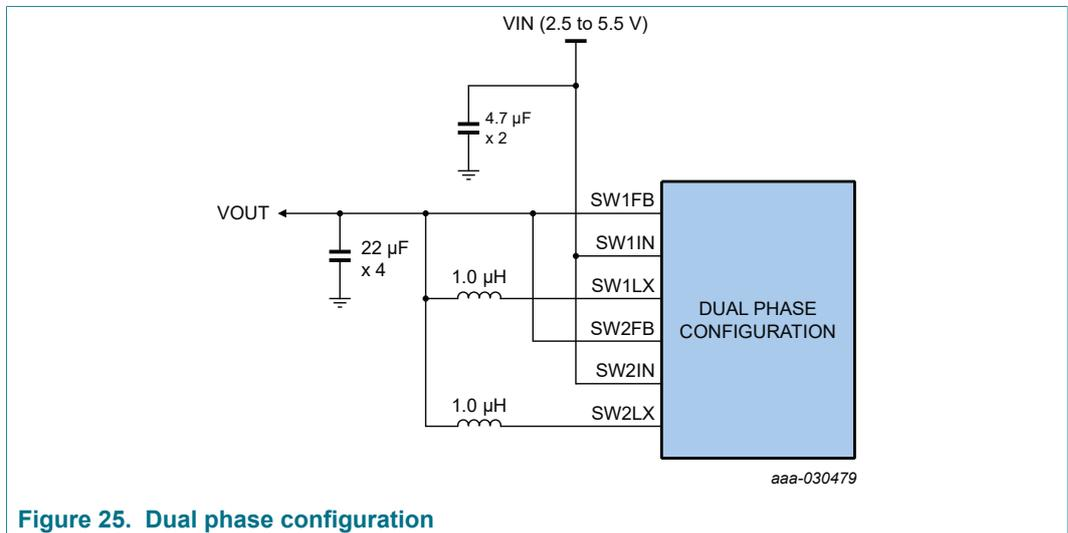
Figure 25. Dual phase configuration
