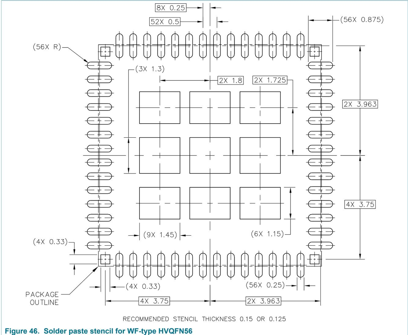
Figure 46. Solder paste stencil for WF-type HVQFN56
