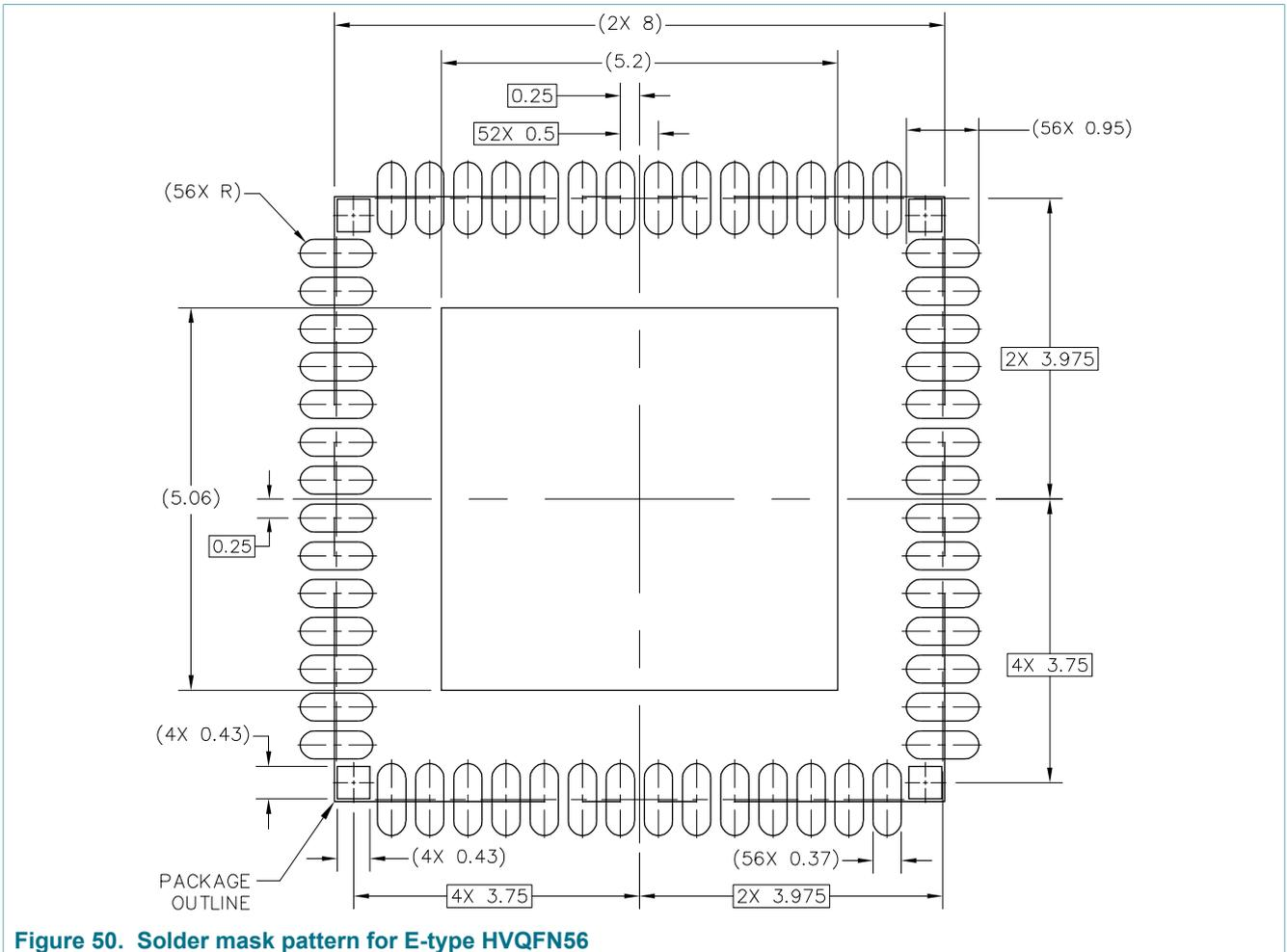
Figure 50. Solder mask pattern for E-type HVQFN56
