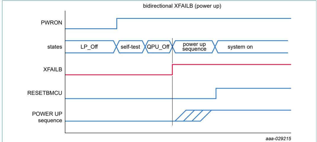
Figure 18. XFAILB behavior during a power up sequence
