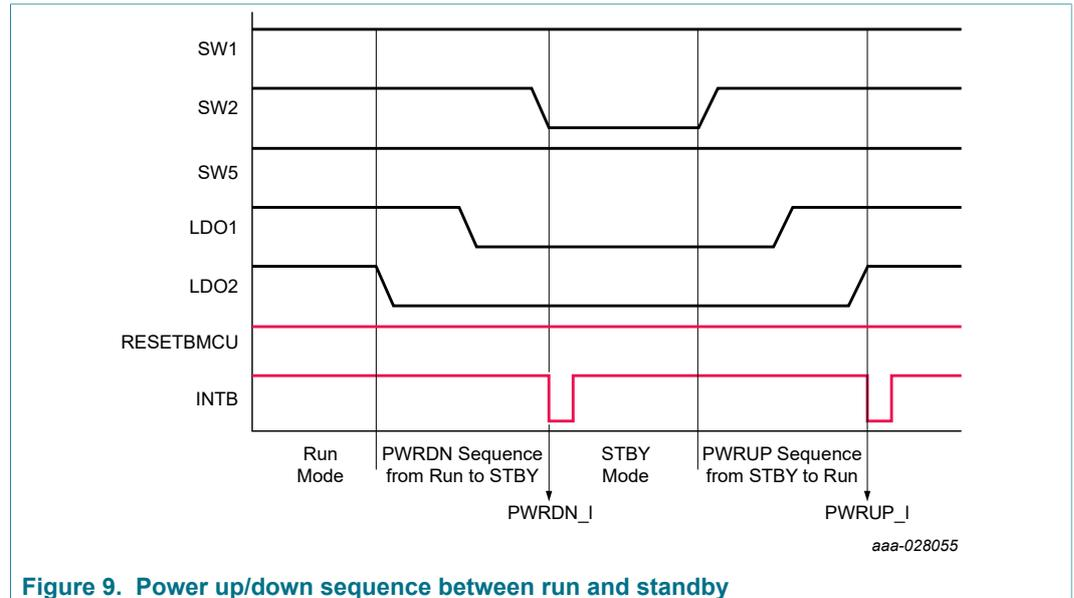
Figure 9. Power up/down sequence between run and standby
