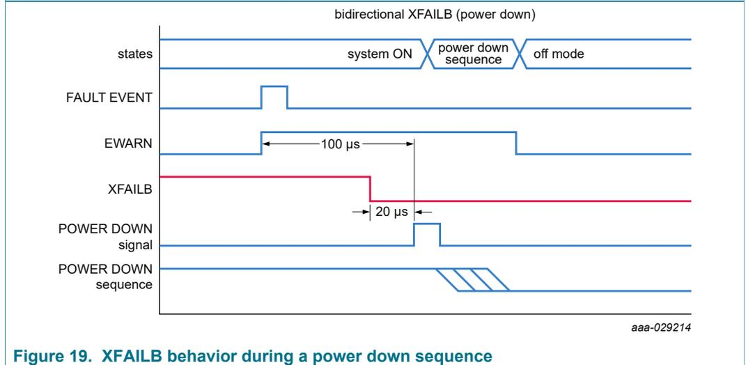
Figure 19. XFAILB behavior during a power down sequence
