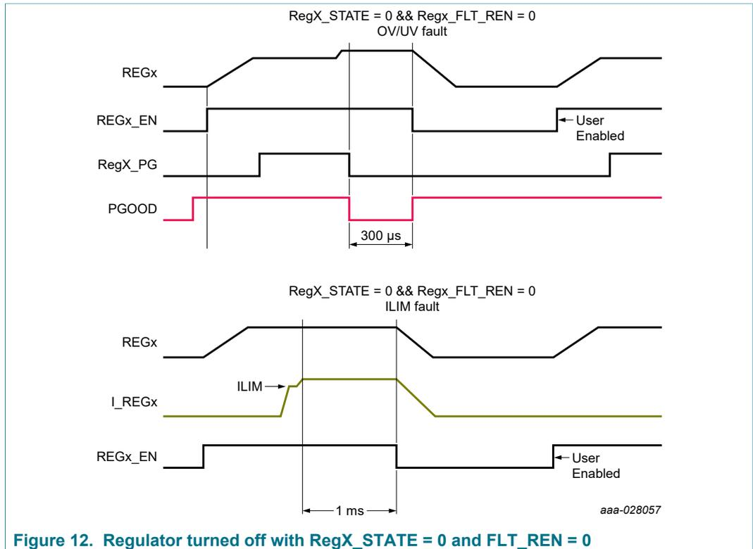
Figure 12. Regulator turned off with RegX\_STATE = 0 and FLT\_REN = 0
