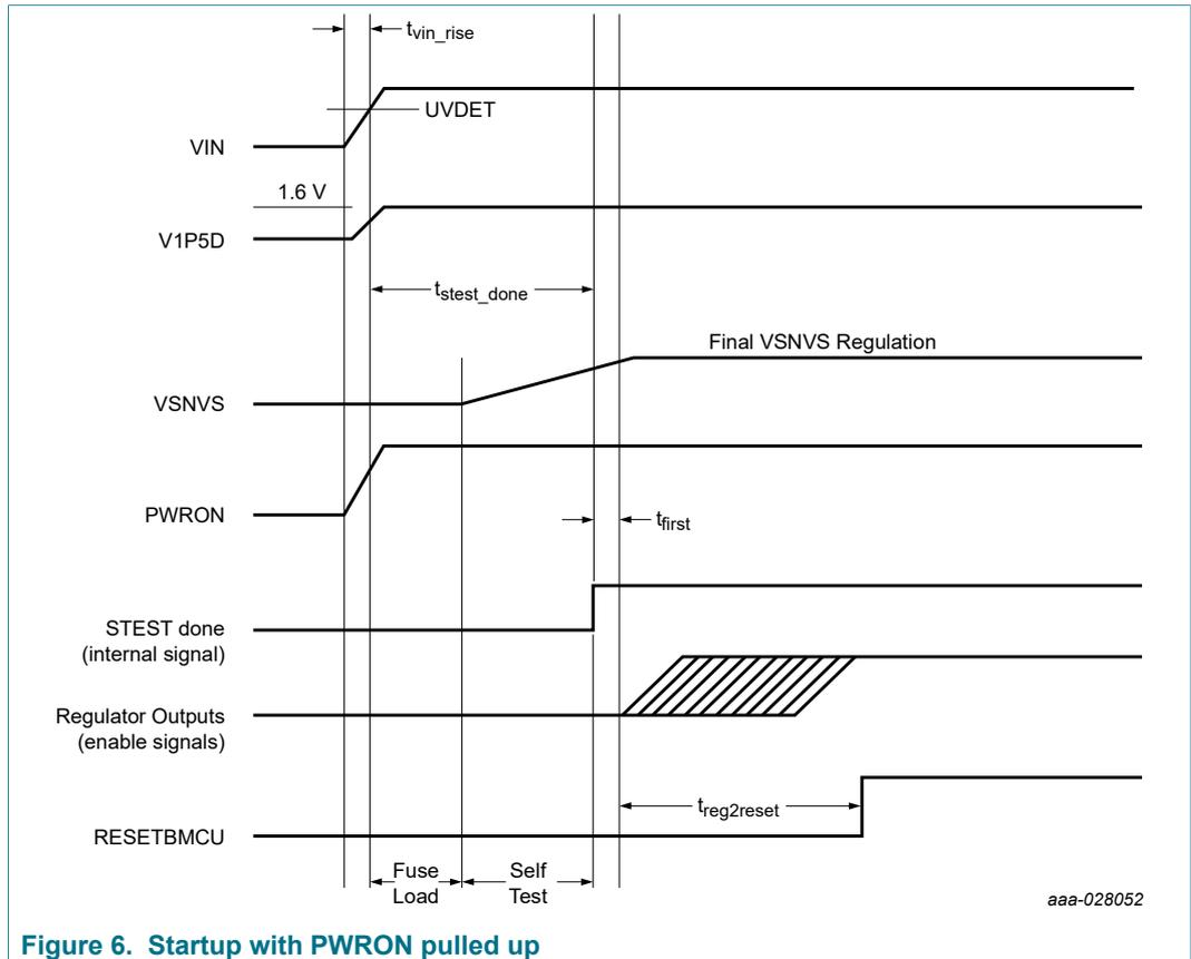
Figure 6. Startup with PWRON pulled up
