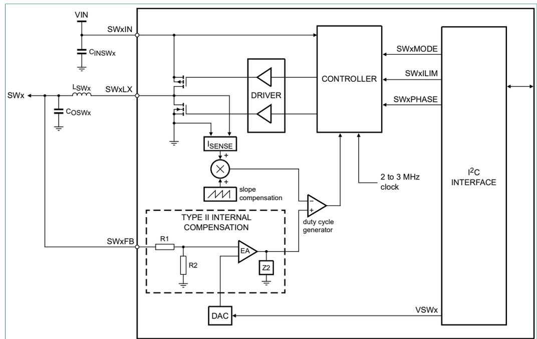
Figure 24. Buck regulator block diagram
