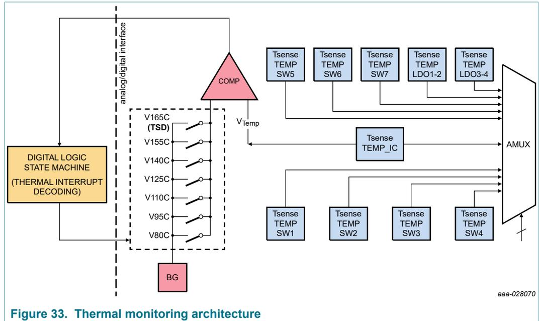
Figure 33. Thermal monitoring architecture
