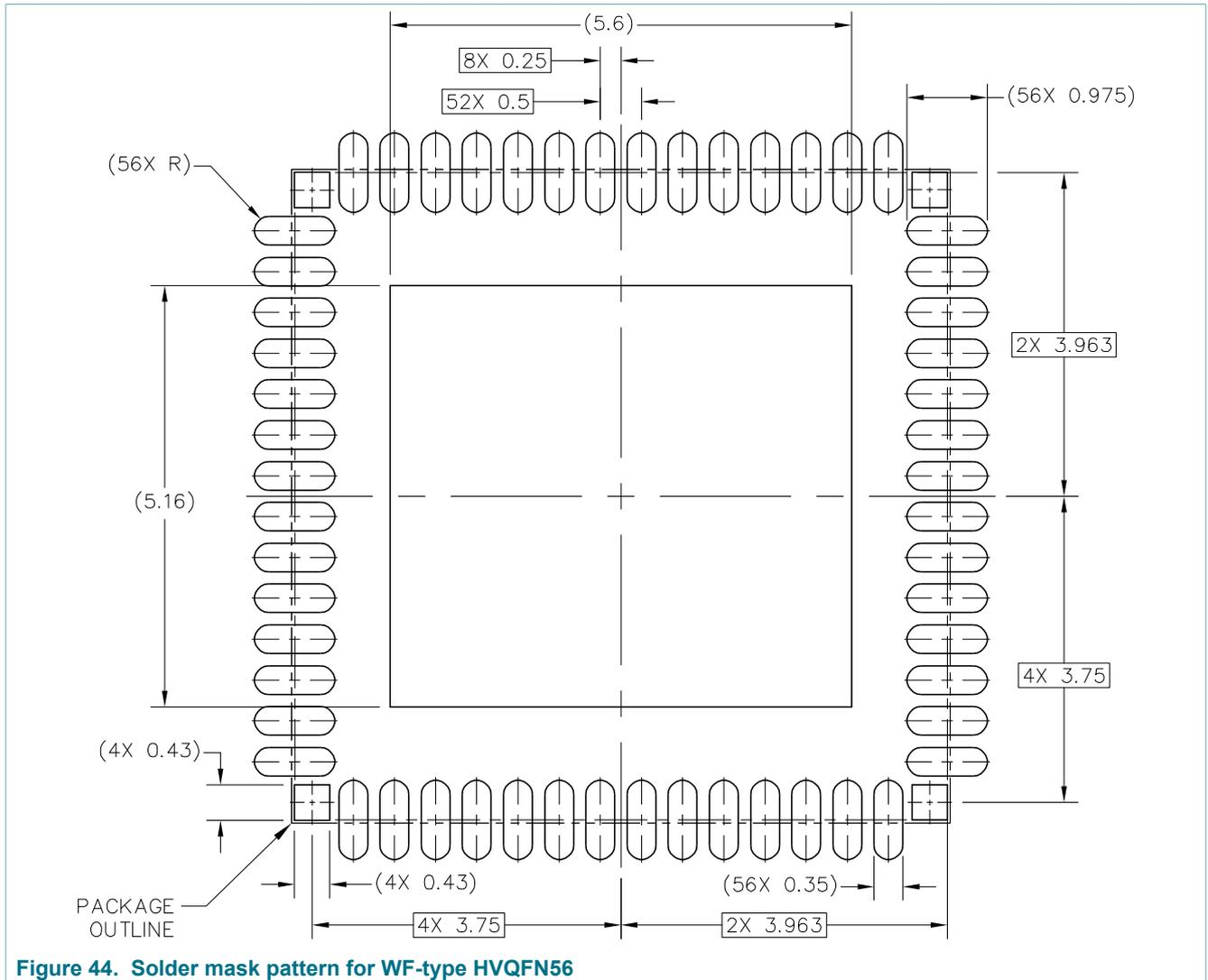
Figure 44. Solder mask pattern for WF-type HVQFN56
