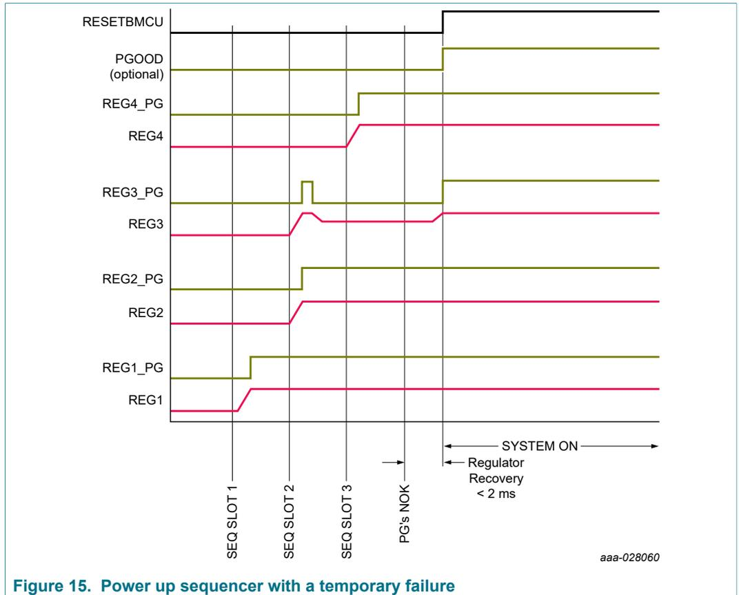
Figure 15. Power up sequencer with a temporary failure
