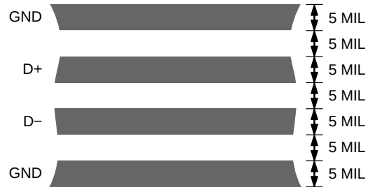
Figure 34. Typical Arrangement of Signal Tracks
