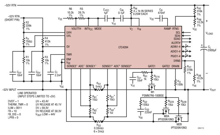
Figure 13. –52V/2500W Hot Swap Controller in Low Stress Staged Start Mode with dV/dt Inrush Control: GATE1 Drives Trickle Startup MOSFET and GATE2 Drives Low R<sub>DS(ON)</sub> MOSFETs, for Systems with Tightly Regulated Supply Voltages
