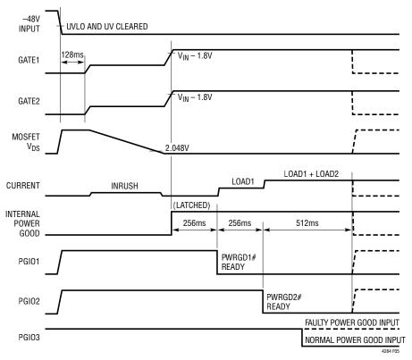
Figure 5. LTC4284 Turn-On Sequence in Parallel Mode
