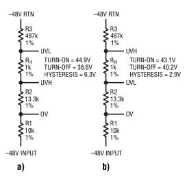
Figure 17. Adjustment of Undervoltage Thresholds for Larger (17a) or Smaller (17b) Hysteresis
