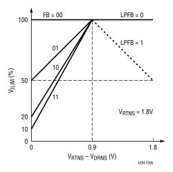
Figure 8b. Current Limit Foldback in Normal Operation
