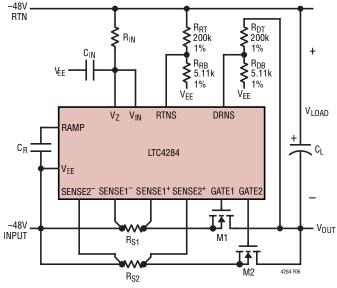
Figure 6. dV/dt Inrush Control Using RAMP Capacitor
