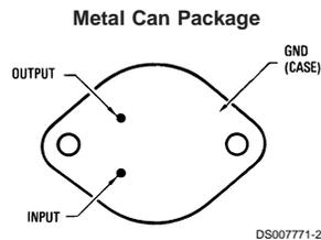
Order Number LM123K STEEL, LM323AK STEEL or LM323K STEEL
