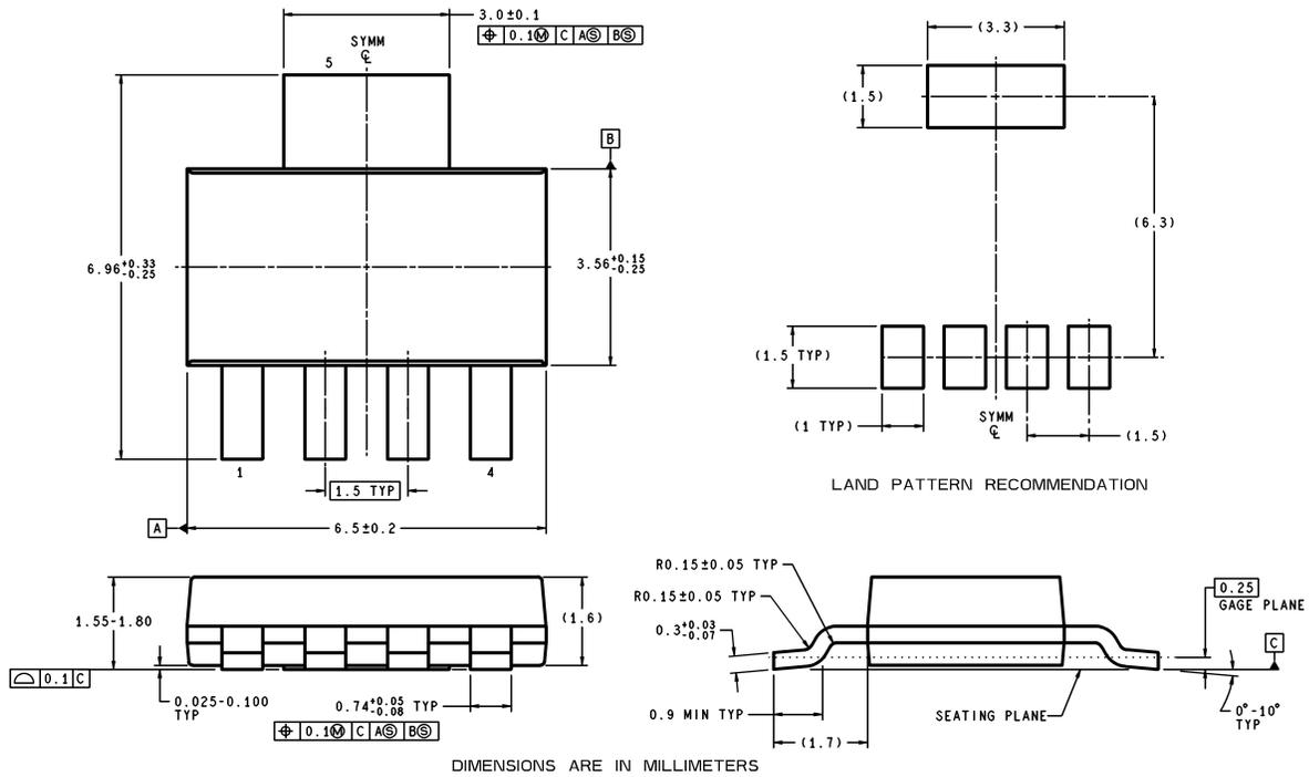
**SOT223, 5-Lead, Molded, Surface Mount Package (SOT223-5)
