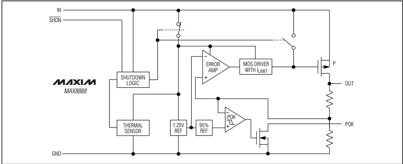
Figure 1. Functional Diagram
