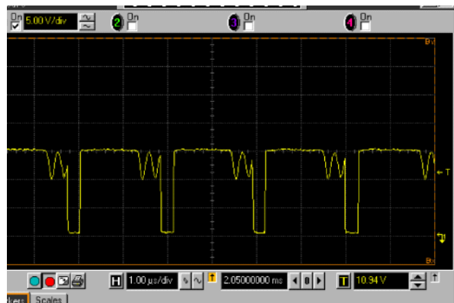
FIGURE 7. BOOST SWITCH NODE AT 100mA (PARTIAL DISCONTINUOUS)
