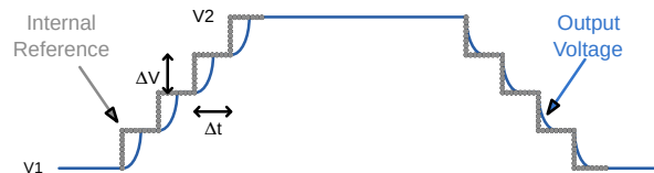
Figure 44. DVS in Forced PPWM Mode Diagram
