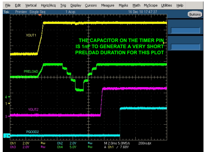
FIGURE 13. NORMAL POWER-UP SEQUENCE
