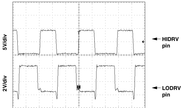
Switching Waveforms, 9A Load
