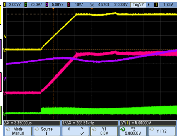
Figure 22. Start-Up Transition at 6A Load
