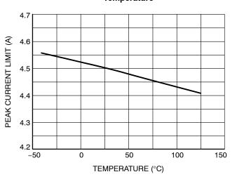
Figure 13. Peak Current Limit vs. Junction Temperature
