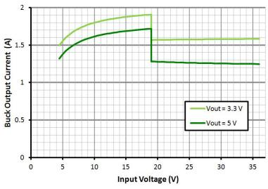
Figure 30. NCV891130 Load Current Capability with a 2.2 μH Inductor
