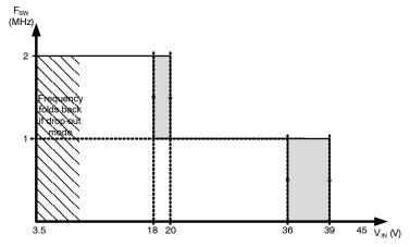
Figure 29. NCV891130 Switching Frequency Profile vs. Input Voltage
