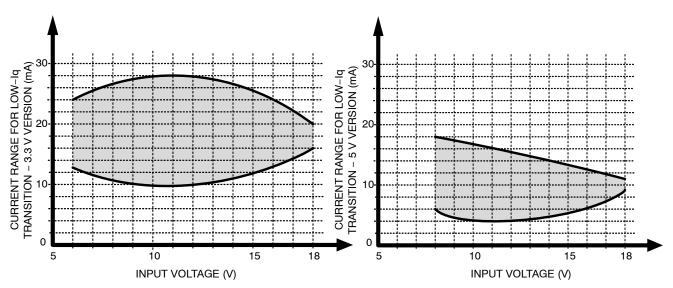
Figure 27. Switcher to Low-Iq Mode Transition (3.3 V Version, 2.2  $\mu$ H) vs. Input Voltage
