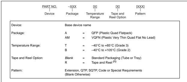
Note 1: Tape and Reel identifier only appears in the catalog part number description. This identifier is used for ordering purposes and is not printed on the device package. See "Orderable Part Numbers" below or check with your Microchip Sales Office for package availability with the Tape and Reel option.
