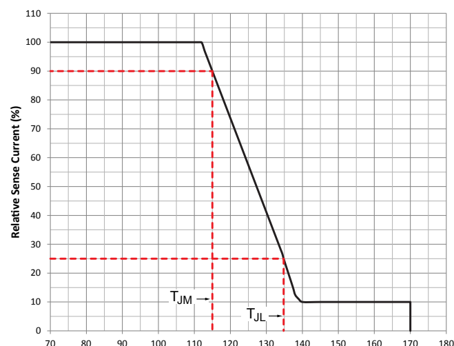
Figure 2. Temperature monitor current reduction.
