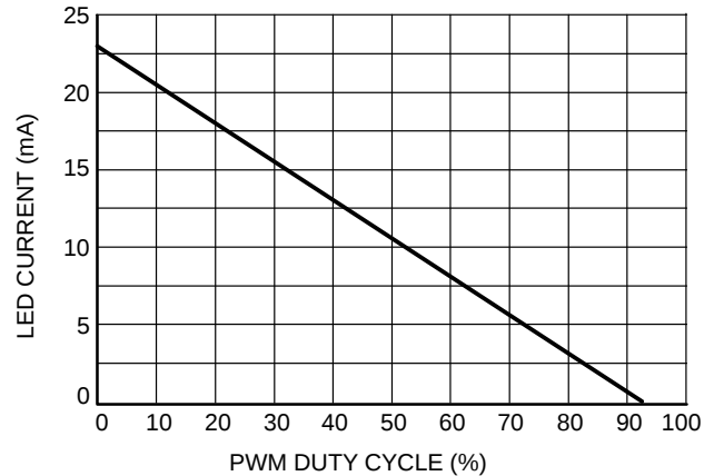
Figure 25. Filtered PWM Dimming (0 V to 2.5 V)
