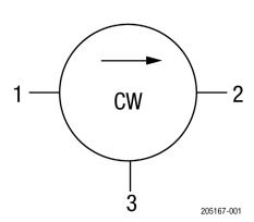
Figure 1. SKYFR-001657 Block Diagram
