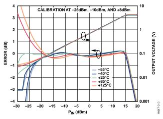
Figure 12. Conformance Error and Output Voltage ( $V_{OUT}$ ) vs. RF Input Power ( $P_{IN}$ ) for Various Temperatures at 1 GHz
