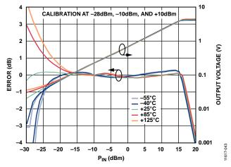
Figure 43. Conformance Error and Output Voltage vs. RF Input Power ( $P_{IN}$ ) and Temperature ( $-55^{\circ}$ C,  $-40^{\circ}$ C,  $+25^{\circ}$ C,  $+85^{\circ}$ C,  $+125^{\circ}$ C) at 10 GHz Using Three Point Calibration
