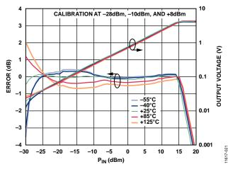
Figure 20. Conformance Error and Output Voltage ( $V_{OUT}$ ) vs. RF Input Power ( $P_{IN}$ ) for Various Temperatures at 25 GHz
