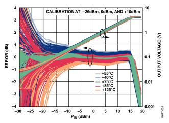
Figure 27. Distribution of Conformance Error with Respect to Output Voltage  $(V_{OUT})$  at 25°C vs. RF Input Power (P<sub>IN</sub>) for Various Temperatures at 30 GHz
