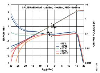
Figure 44. 10 GHz Conformance Error and Output Voltage vs. RF Input Power (P<sub>IN</sub>) for Second Device at +25°C, −40°C, −55°C, +85°C, and +125°C
