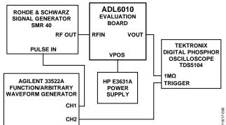
Figure 37. Hardware Configuration for Output Response to RF Burst Input Measurements
