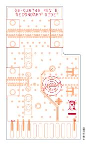
Figure 49. ADL6010 Evaluation Board Layout, Bottom Side
