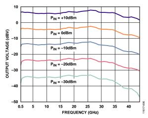
Figure 5. Output Voltage (V<sub>OUT</sub>) Flatness vs. Frequency for Five RF Input Power Values (P<sub>IN</sub>)
