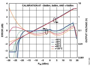
Figure 29. Conformance Error and Output Voltage ( $V_{OUT}$ ) vs. RF Input Power ( $P_{IN}$ ) for Various Temperatures at 43.5 GHz
