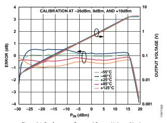
Figure 24. Conformance Error and Output Voltage ( $V_{OUT}$ ) vs. RF Input Power ( $P_{IN}$ ) for Various Temperatures at 30 GHz
