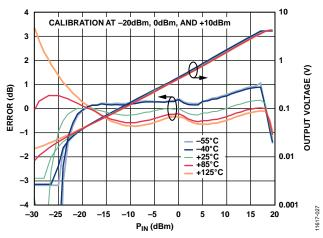
Figure 26. Conformance Error and Output Voltage ( $V_{OUT}$ ) vs. RF Input Power ( $P_{IN}$ ) for Various Temperatures at 40 GHz
