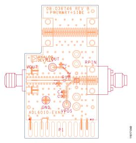
Figure 48. ADL6010 Evaluation Board Layout, Top Side
