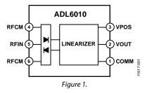
topology is that no even-order distortion, caused by nonlinear source loading, occurs at the input. This is an important benefit in applications where a low ratio coupler is used to extract a signal sample and is a significant improvement over traditional diode detectors.
