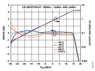
Figure 19. Conformance Error and Output Voltage ( $V_{OUT}$ ) vs. RF Input Power ( $P_{IN}$ ) for Various Temperatures at 20 GHz
