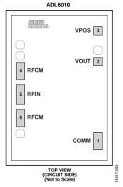
Figure 3. 6-Pad Bare Die Pin Configuration
