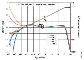
Figure 42. Conformance Error and Output Voltage vs. RF Input Power ( $P_{IN}$ ) for Various Temperatures ( $-55^{\circ}$ C,  $-40^{\circ}$ C,  $+25^{\circ}$ C,  $+85^{\circ}$ C, and  $+125^{\circ}$ C) at 10 GHz Using Two Point Calibration
