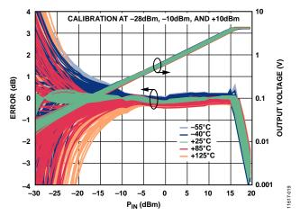
Figure 21. Distribution of Conformance Error with Respect to Output Voltage  $(V_{OUT})$  at 25°C vs. RF Input Power (P<sub>IN</sub>) for Various Temperatures at 15 GHz
