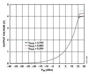
Figure 6. Output Voltage (V<sub>OUT</sub>) vs. RF Input Power (P<sub>IN</sub>) for Various Supply Voltages
