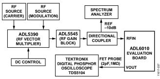
Figure 39. Hardware Configuration for Envelope Output Response Measurement
