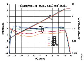
Figure 25. Conformance Error and Output Voltage ( $V_{OUT}$ ) vs. RF Input Power ( $P_{IN}$ ) for Various Temperatures at 35 GHz
