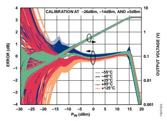
Figure 11. Distribution of Conformance Error with Respect to Output Voltage  $(V_{OUT})$  at 25°C vs. RF Input Power ( $P_{IN}$ ) for Various Temperatures at 0.5 GHz
