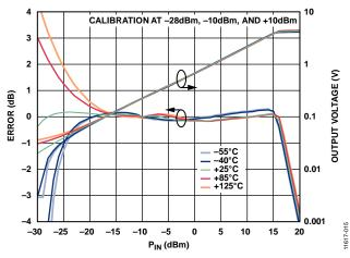
Figure 14. Conformance Error and Output Voltage ( $V_{OUT}$ ) vs. RF Input Power ( $P_{IN}$ ) for Various Temperatures at 10 GHz
