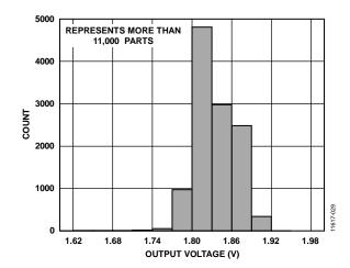
Figure 31. Output Voltage (V<sub>OUT</sub>) Distribution,  $P_{IN} = 9 \, dBm$  at 12 GHz, 25°C
