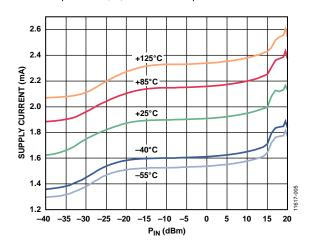
Figure 9. Supply Current vs. RF Input Power (P<sub>IN</sub>) for Various Temperatures
