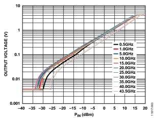
Figure 4. Typical Output Voltage (V<sub>OUT</sub>) vs. RF Input Power (P<sub>IN</sub>) at Various Frequencies (0.5 GHz to 43.5 GHz) at 25°C
