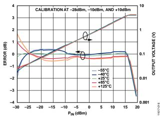
Figure 18. Conformance Error and Output Voltage ( $V_{OUT}$ ) vs. RF Input Power ( $P_{IN}$ ) for Various Temperatures at 15 GHz
