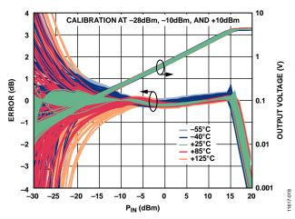
Figure 17. Distribution of Conformance Error with Respect to Output Voltage  $(V_{OUT})$  at 25°C vs. RF Input Power (P<sub>IN</sub>) for Various Temperatures at 10 GHz
