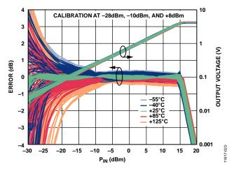
Figure 22. Distribution of Conformance Error with Respect to Output Voltage (V<sub>OUT</sub>) at 25°C vs. RF Input Power (P<sub>IN</sub>) for Various Temperatures at 20 GHz
