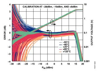
Figure 23. Distribution of Conformance Error with Respect to Output Voltage (Vout) at 25°C vs. RF Input Power (PIN) for Various Temperatures at 25 GHz
