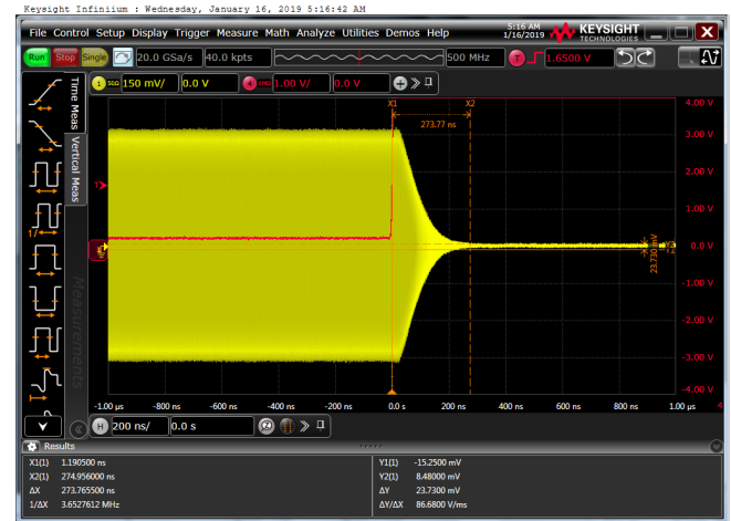
Figure 24. RX Mode to Standby Transient Time
