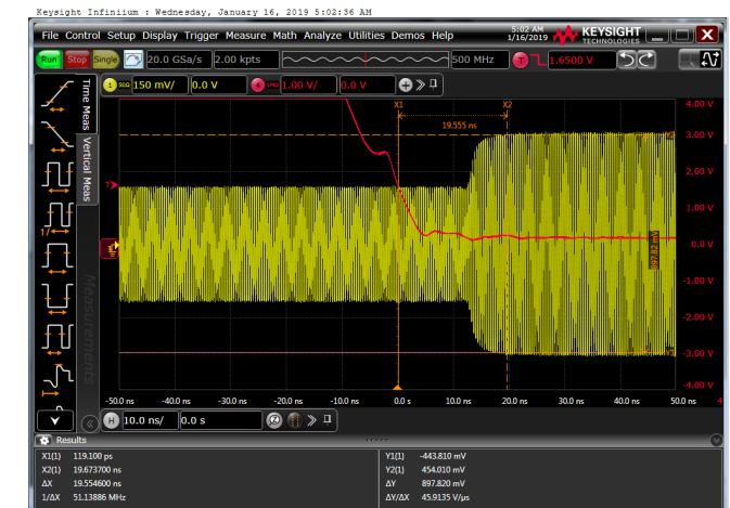
Figure 26. 6dB Gain Increase Transient Time
