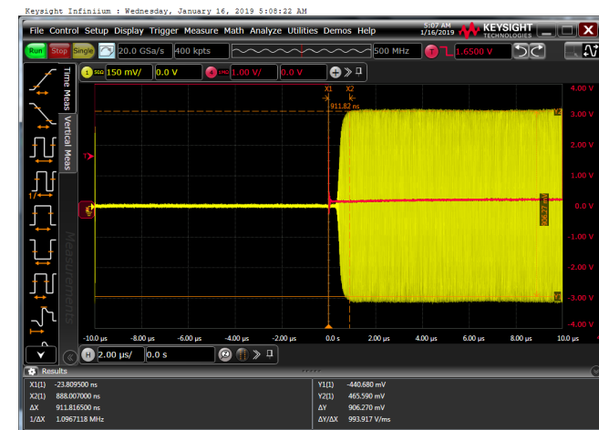
Figure 25. 6dB Gain Reduction Transient Time
