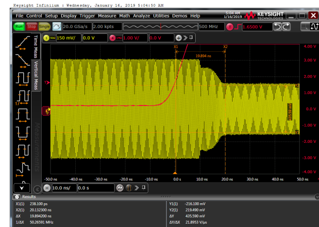
Figure 25. 6dB Gain Reduction Transient Time
