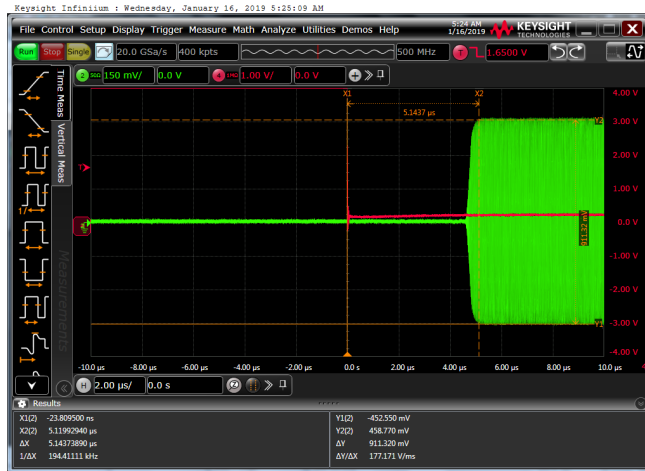
Figure 23. Standby to RX Mode Transient Time
