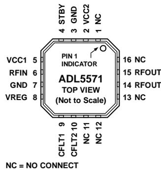
Figure 2. Pin Configuration
