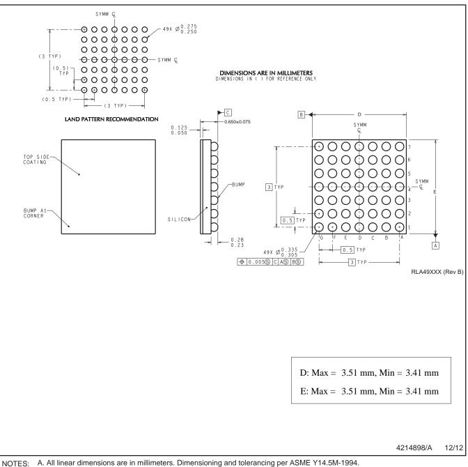
IOTES: A. All linear dimensions are in millimeters. Dimensioning and tolerancing per ASME Y14.5M-1 B. This drawing is subject to change without notice.
