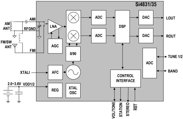
Figure 2. Si4831/35-B30 Functional Block Diagram
