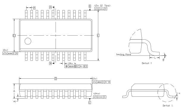
Figure 3. 24-Pin SSOP
