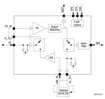
Figure 1. SKY66122-11 Functional Block Diagram
