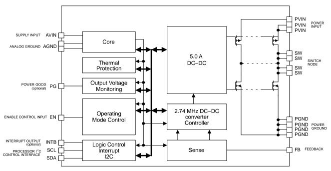
Figure 2. Simplified Block Diagram
