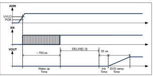
Figure 33. Initial Power Up Sequence
