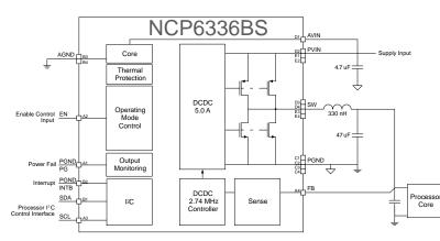
Figure 1. Typical Application Circuit
