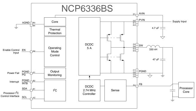
Figure 46. Typical Application Schematic
