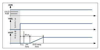
Figure 36. Fast Power Up Sequence
