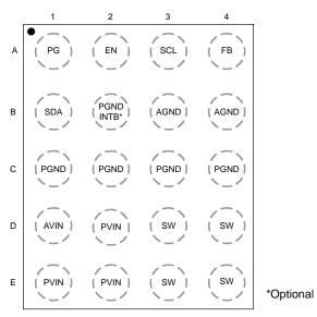
Figure 3. Pin Out (Top View)
