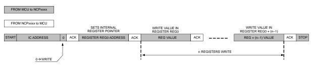
Figure 45. Write in n Registers
