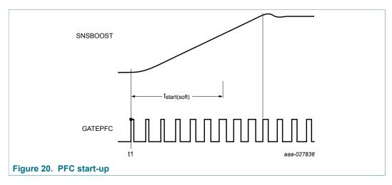
At t1, all conditions to start up the PFC are fulfilled. When the PFC starts switching, the maximum on-time is increased cycle-by-cycle from zero until the  $t_{\text{on}}$  regulation limits the on-time of the PFC external MOSFET.
