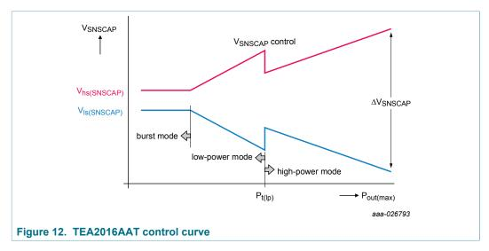
When the output power ( $P_{out}$ ) is at its maximum, the low capacitor voltage level ( $V_{ls(SNSCAP)}$ ) is at its minimum and the high capacitor voltage ( $V_{hs(SNSCAP)}$ ) is at its maximum level. According to Equation 1 in Section 8.2, the maximum  $\Delta V_{SNSCAP}$  ( $V_{hs(SNSCAP)} - V_{ls(SNSCAP)}$ ), which is the divided  $\Delta V_{Cr}$  voltage, corresponds to the maximum output power.
