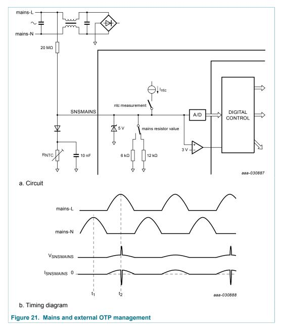
The TEA2016AAT continuously measures the SNSMAINS voltage via an A/D converter and waits until it detects a peak (t1). This peak value is internally stored and used as an input for the brownout/brownin detection and the mains compensation.
