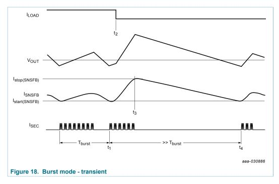
At t1, the system starts with a new burst cycle period. Shortly later at t2, the output load is reduced. As a result the output voltage shows an overshoot and the optocoupler current increases. To limit the overshoot, the system also ends the burst cycle when the optocoupler current exceeds the  $I_{\text{stop(burst)}}$  level.
