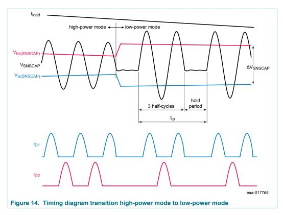
As the system continuously tracks the primary capacitor voltage, it knows exactly when to enter the "hold" period. It can also continue again at exactly the correct voltage and current levels of the resonant converter. In this way, a "hold" period can be introduced which reduces the magnetization and switching losses without any additional losses. The currents  $I_{D1}$  and  $I_{D2}$  (see Figure 14) are the secondary currents through diodes D1 and D2 (see Figure 25).
