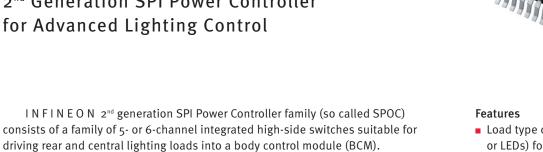
The SPOC II family, scaled by number of channels and features (basic, LED mode, cranking), addresses this trend and integrates multiple channels inside one package to reduce board space. SPOC II devices feature a serial peripheral interface (SPI), enabling customers to save I/Os in the microcontroller and reduce the amount of external components required for a discrete implementation. The LED mode in BTS5672E and BTS5682E is programmable via SPI.
