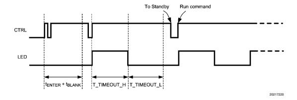
LED OFF time counter can saturate also if Training end command is not given or no new ON time has been started. In this case saturated OFF time is recorded and chip goes to Standby.
