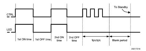
If Training End command is introduced during LED ON time capturing, the associated LED ON period is not recorded and hence neither OFF time. Notice that valid OFF time before Training End is longer than half of Minimum LED OFF period (T\_CYCLE\_L).
