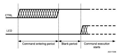
If CTRL signal is low after command entering period, command execution starts when CTRL is pulled high. This does not apply to Run command. With Run command CTRL must be high. Note that no rising edges are allowed during blank period.
