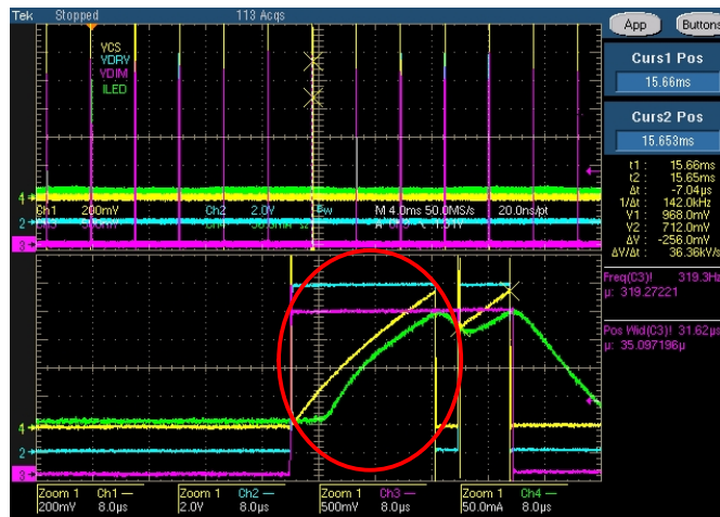
Figure 31. Minimum Dimming Duty Cycle
