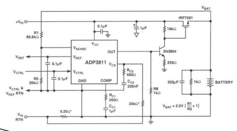
Figure 29. ADP3811 Controlling a Linear Battery Charger
