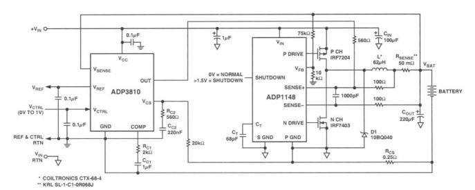
Figure 28. High Efficiency Buck Battery Charger
