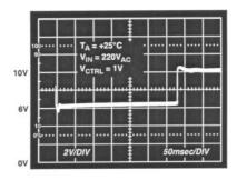
Figure 27. Output Voltage Transient Response to Battery Connect/Disconnect
