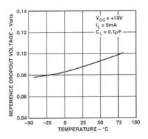
Figure 2. Reference Output Voltage Temperature for Two Typical Parts
